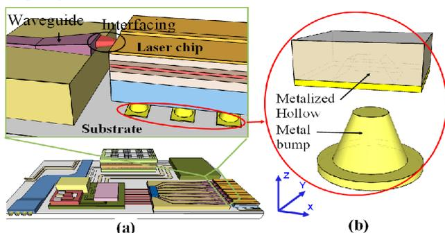
Fig. 1 Electronics-optics heterogeneously integrated module (a) and proposed gold to gold interconnection (b).
