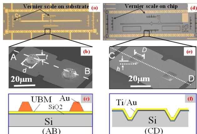
Fig. 3 Fabricated substrate (left) and chip (right) samples. Zoom-in images show the Au bump (b) and Au-deposited hollow pyramid (e).  $d = 10 \mu\text{m}$ ,  $t = 6 \mu\text{m}$ ;  $D = 12 \mu\text{m}$ ,  $h = 4 \mu\text{m}$ . (c), (f) are the sketch of cross-section views of these elements.
