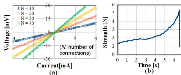
Fig. 5 I-V characteristic of the bonding interconnection (a), and shear bond strength test result (b).
