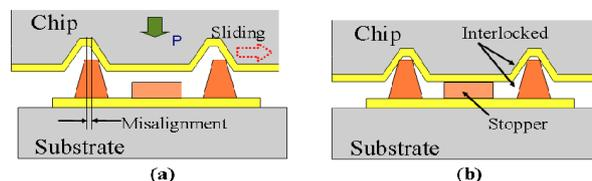
Fig. 2 Drawings show the working principle of proposed misalignment self-correction pair structure. Bump and hollow structures provide mechanical guides for maintaining high precision alignment between the interconnect pads during the bonding process.
