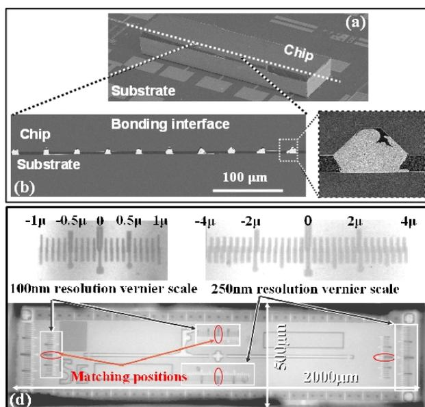
Fig. 4 Images of a typical bonded chip. Force of 15 N, along with ultrasonic energy of 48.5 kHz wave, amplitude of 2.2  $\mu\text{m}$  activated in 500 ms, were applied at ambient temperature. (a) is the bird's-eye view of the chip on substrate; (b) is the cross-section view at bonding interface; (c) is the IR images showing the micro vernier, illustrating the bonding tolerance, confirming the self-correction function of truncated cone bump and hollow concave structures after bonding process.
