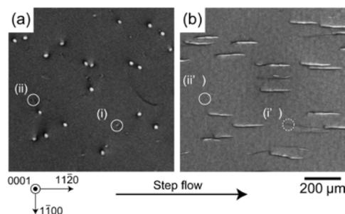
Figure 2. X-ray topography images taken before (a) and after (b) solution growth on the vicinal 4H-SiC seed crystal. TEDs which are imaged as small circular contrast were converted to BPDs imaged as linear contrast as (i) and (i') for example, while the other TEDs were propagated as (ii) and (ii') for example.
