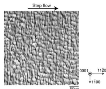
Figure 1. DIC image taken from the grown crystal on a vicinal seed crystal.
