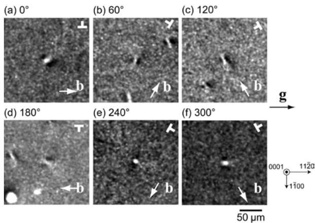
Figure 3. X-ray topography images of TEDs taken before solution growth. (a)-(f) correspond to the six TEDs with different Burgers vectors and angle between the step-flow direction and the Burgers vectors ( $\theta$ ) is  $0^\circ$ ,  $60^\circ$ ,  $120^\circ$ ,  $180^\circ$ ,  $240^\circ$  and  $300^\circ$ , respectively.
