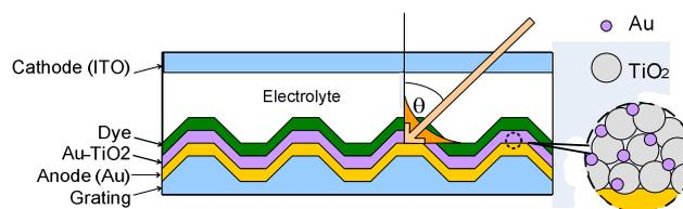
Fig. 1 Fabricated dye-sensitized solar cells (DSSCs)
