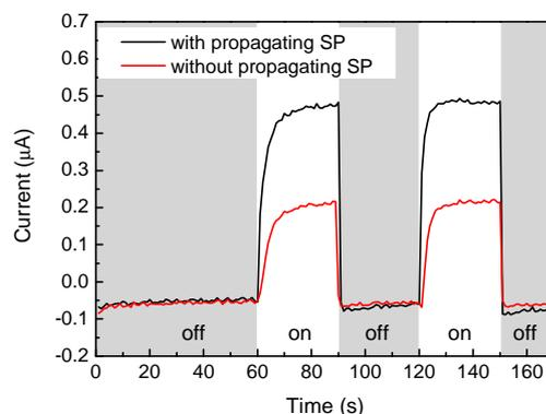
Fig. 2 Short-circuit photocurrent properties of the dye-sensitized cell composed of the Au grating/ Au-TiO<sub>2</sub>/TMPyP-SCC LbL (20 bilayers)/electrolyte/ITO substrate upon irradiation of visible light with surface plasmon excitation (p-pol.) and without surface plasmon excitation (s-pol.).
