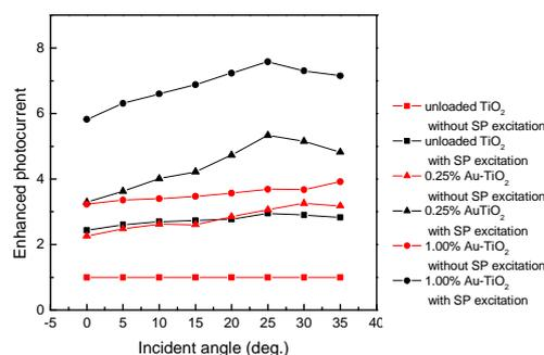
Fig. 3 Enhanced photocurrent factor, that is, the ratio of the current of all samples to the current with unloaded TiO<sub>2</sub> without propagating SP excitation, as a function of the incident light angle.
