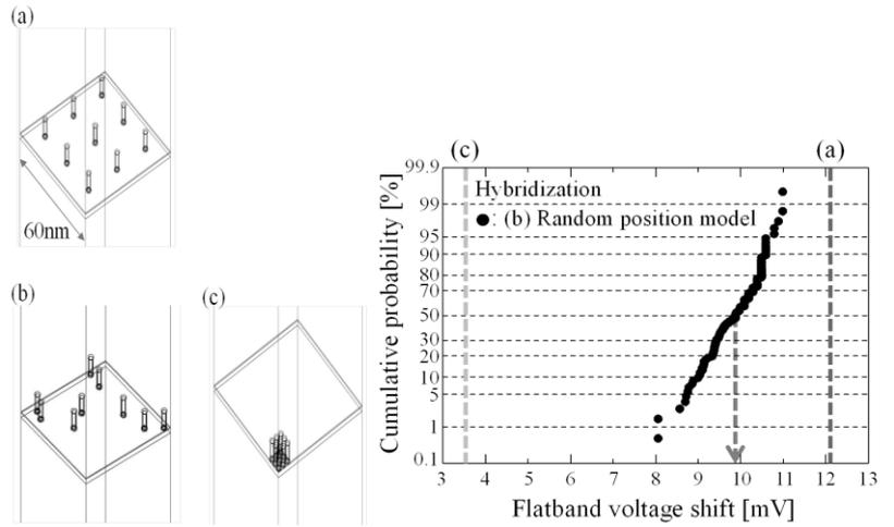
Fig. 4 Influence on flatband voltage shift due to position of upright DNA.
