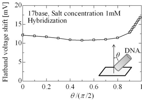
Fig. 5 Influence on flatband voltage shift due to DNA orientation angle  $\theta$ .
