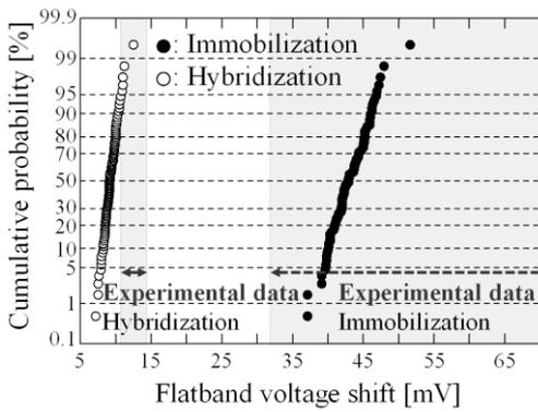
Fig. 3 Flatband voltage shift due to DNA whose position and orientation are random. In experiment, threshold voltage shift is 32~100mV at Immobilization, 11~14mV at Hybridization [5-7].
