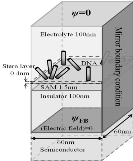
Fig. 1 Schematic illustration of ion-sensitive field-effect transistor (ISFET) model.
