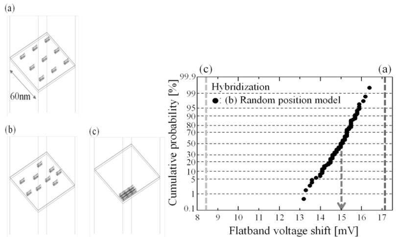
Fig. 6 Influence on flatband voltage shift due to position of DNA tilted 90 degrees. (a) Ordered position model ( $\Delta V_{FB} = 17.1\text{mV}$ ), (b) Random position model (median  $\Delta V_{FB} = 15.0\text{mV}$ ), (c) Dense position model ( $\Delta V_{FB} = 8.41\text{mV}$ ).
