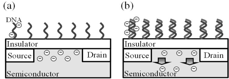
Fig. 2 Principle of DNA detection by ISFET.
