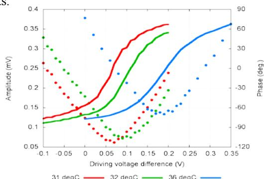
Fig. 2 OPBS-based amplitude (dots) and phase (lines) signals for water solution at three temperatures.
