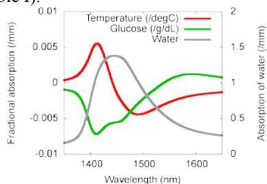
Fig. 3 Spectroscopic data of fractional absorption coefficients of glucose and temperature, and comparison with water absorption.
