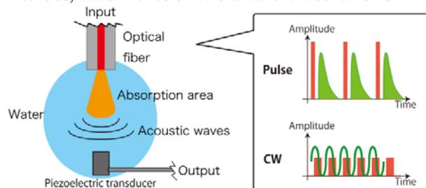
Fig. 1 Schematic view of CW-PA basic concept (left) with the two main excitation sequence: pulse and CW (right).
