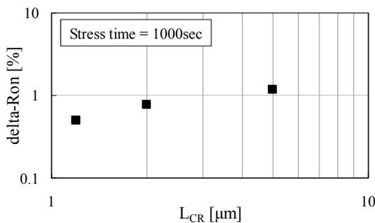
Fig. 5  $L_{CR}$  dependence of  $\Delta R_{on}$  shift in pLDMOS.
