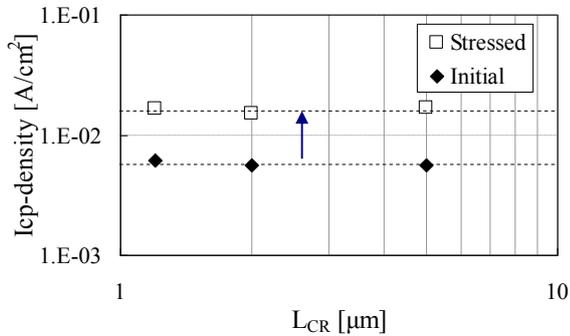
Fig. 4  $L_{CR}$  dependence of  $I_{cp}$ -density shift on CR in pLDMOS.
