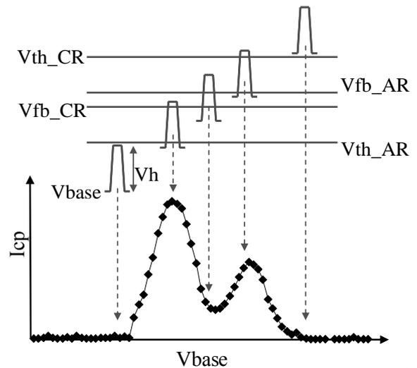
Fig. 2 Schematic illustration of  $I_{cp}$  measurement method for LDMOS transistors. This shows relationship between pulse, threshold voltage ( $V_{th}$ ) and flat-band voltage ( $V_{fb}$ ) for CR and AR. Amplitude of pulse ( $V_h$ ) on  $I_{cp}$  measurement is constant
