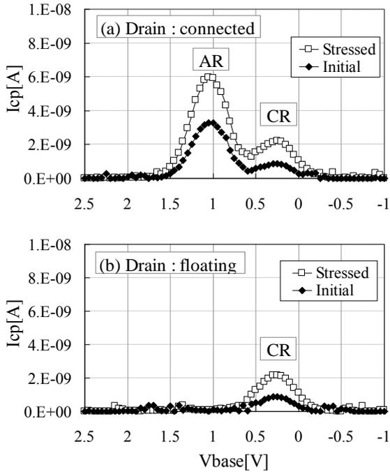
Fig. 3 Typical  $I_{cp}$  curves measured with (a) drain connected to VSS and (b) drain left floating in pLDMOS.
