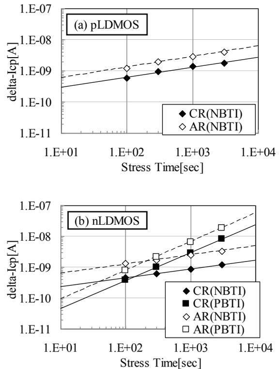
Fig. 6  $\Delta I_{cp}$  shifts in (a) pLDMOS and (b) nLDMOS under NBTI and PBTI stress.
