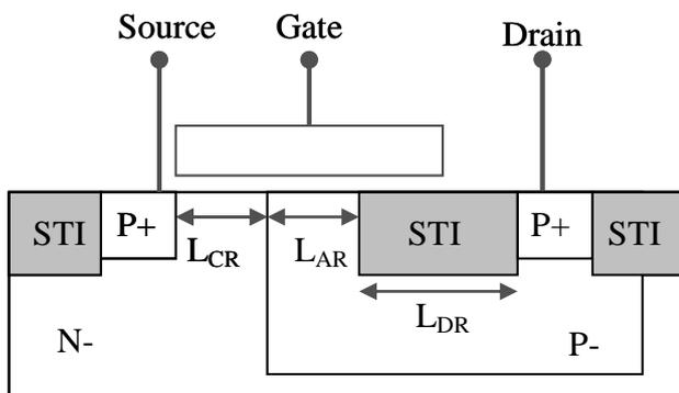
Fig. 1 Cross section of pLDMOS.
