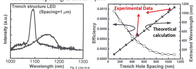
Fig. 2. The electroluminescence spectra from Si LED with and without nm-scale textured surface structure. The high light emission intensity enhancement and obvious photonic crystal effect to extract the special light emission wavelength are observed.
