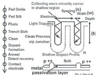
Fig. 1. The schematic diagram of the nm-scale trench structure for the application of Si LED and solar cell.
