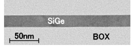
Fig.7 TEM image of cross section of H^+ ion implanted SiGe layer with R of 55%, where E_A = 10 \text{ keV} and D_I = 1 \times 10^{17} \text{ cm}^{-2} . We have observed no dislocations.
