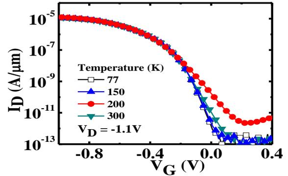
Fig.5 ID-V<sub>G</sub> curves of TFET fabricated by plasma implantation and laser annealing at different temperatures. (The curve shift with temperature has been accounted by shifting the curve to same V<sub>G</sub> at 10<sup>-7</sup>A/μm)
