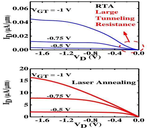
Fig. 4 The ID-VD curve of TFETs fabricated by (a) RTA and (b) laser annealing.
