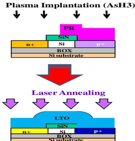
Fig. 2 Parts of process flow of TFET fabricated with laser annealing.
