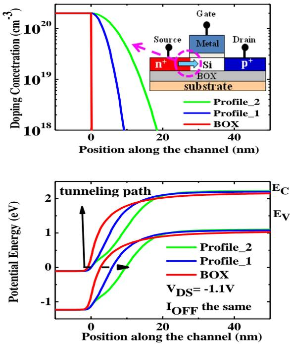
Fig. 1 (a) The device structure of Si n-i-p TFET with different lateral n<sup>+</sup> source doping profiles. (L<sub>g</sub>=100nm, EOT=1nm, channel doping=1e16cm<sup>-3</sup>, T<sub>Si</sub>=50nm) (b) Simulated band diagrams of TFETs with different lateral source doping profiles.
