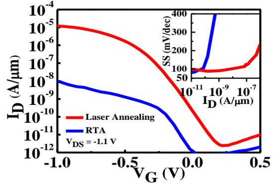
Fig. 3 The subthreshold characteristics of Si TFETs fabricated by plasma implantation and different annealing methods.
