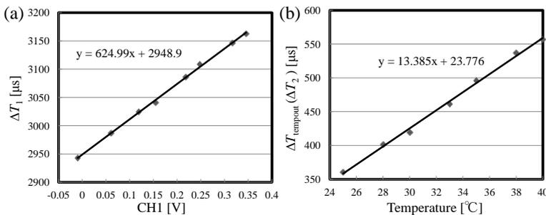
Fig. 7 Wireless measurement using dual data PWM. (a) Result of external input CH1. (b) Result of temperature measurement.
