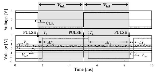
Fig. 4 Measurement result of dual data PWM circuit. The pulse width  $\Delta T_1$  and  $\Delta T_2$  is changed in proportion to independent signal  $V_{in1}$  and  $V_{in2}$ , respectively.
