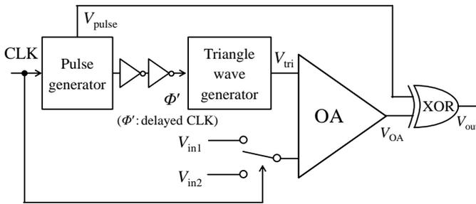
Fig. 3 Block diagram of dual data PWM circuit that consist of pulse generator, triangle wave generator, OA, and XOR.
