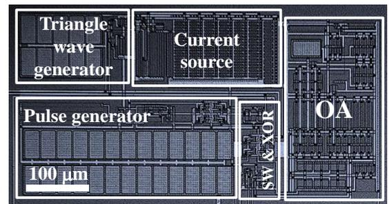
Fig. 8 Micrograph of dual data PWM circuit.
