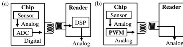
Fig. 1 (a) Block diagram of conventional RFID biosensor. (b) Block diagram of RFID biosensor with PWM.
