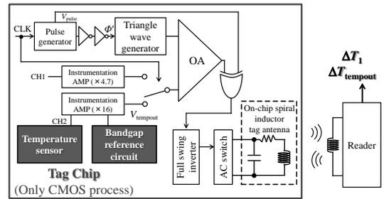
Fig. 6 Block diagram of wireless measurement circuit with dual data PWM.
