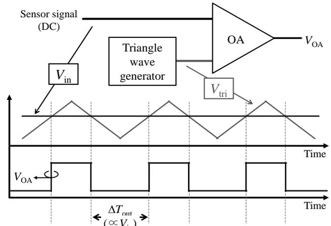
Fig. 2 Basic PWM circuit. The pulse width  $\Delta T_{out}$  is proportional to input signal  $V_{in}$ .
