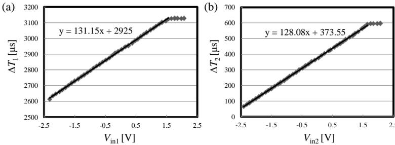
Fig. 5 (a) Measurement result of dual data PWM when  $V_{in1}$  and  $V_{in2}$  are swept in the range from -2.4V to 2.2V. (a)  $\Delta T_1$ . (b)  $\Delta T_2$ .
