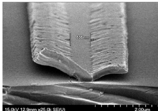
**Fig. 2** Cross-section profile of T-shaped gate with slant sidewall.
