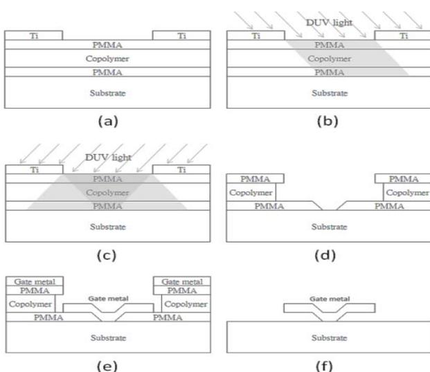
**Fig. 1** Fabrication process of the AlGaIn/GaN HEMT with slant field-plate structure using deep-UV lithography with angle exposure.
