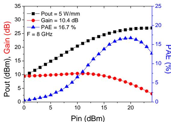
**Fig. 3** Power measurement of the AlGaIn/GaN HEMT with slant gate at 8 GHz.  $V_{GS} = -1.5$  V,  $V_{DS} = 50$  V.
