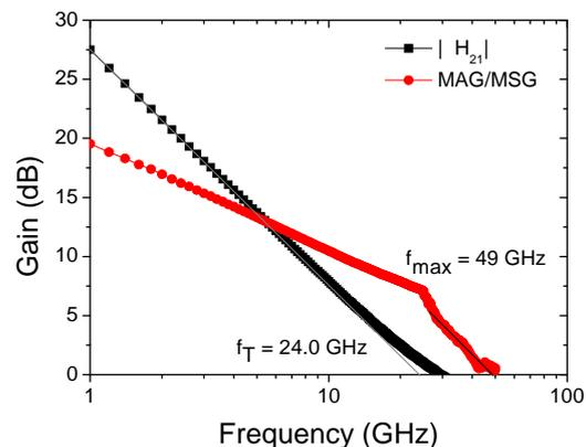
**Fig. 4** RF performance at  $V_{DS} = 10$  V and  $V_{GS} = -1.7$  V for AlGaIn/GaN HEMT. Extrapolation with -20 dB/dec yields  $f_T = 24$  GHz and  $f_{max} = 49$  GHz.
