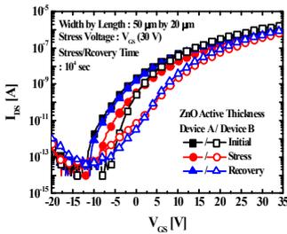
Fig. 1. Transfer characteristic curves of ZnO TFTs before and after stress, and under relaxation.
