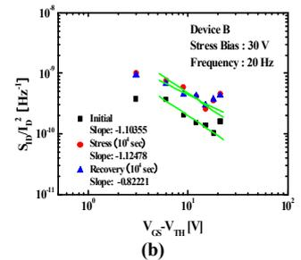
Fig. 3.  $S_{ID}/I_D^2$  according to  $V_{GS}-V_{TH}$  after the stress bias of 30 V for the stress and relaxation time of  $10^4$  sec in ZnO TFTs.
