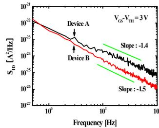
Fig. 2.  $S_{ID}$  according to frequency in ZnO TFTs.
