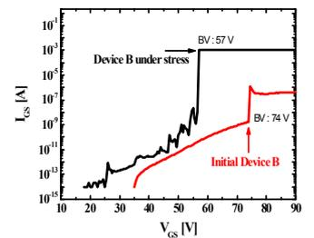
Fig. 6. Breakdown voltage (BV) of device B under stress and initial device B
