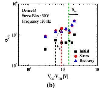
Fig. 4.  $\alpha_{app}$  according to  $V_{GS}-V_{TH}$  under the stress bias of 30 V for the stress and relaxation time of  $10^4$  sec in ZnO TFTs.
