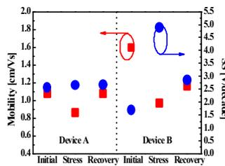
Fig. 5. Mobility and SS of ZnO TFTs before and after stress, and under relaxation.
