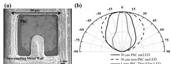
Fig. 2 (a) GaN-based  $30 \mu\text{m}$  mcLED with 2D square lattice of circular PhC holes of  $a=370$  nm, and  $t=80$  nm PhCs, and (b) far-field emission distributions of devices as well as the prior study in deep-PhC ( $t=250$  nm) thin-film LED with chip size as  $1\text{mm} \times 1\text{mm}$ .
