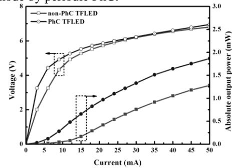
Fig. 4 The output power-current-voltage characteristics of mcLED with and without PhC.
