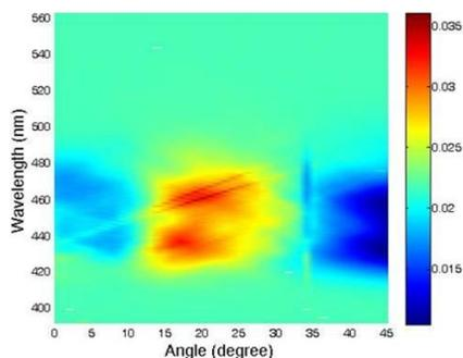
Fig. 3 Angular-resolved spectra without polarizer for  $30 \mu\text{m}$  PhC mcLED.
