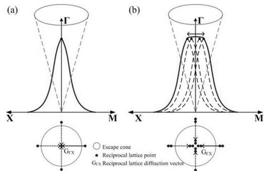
Fig. 1 Diffraction profile accompanied reciprocal lattice of PhC with (a)  $\Gamma$ -point and (b) near- $\Gamma$  points.
