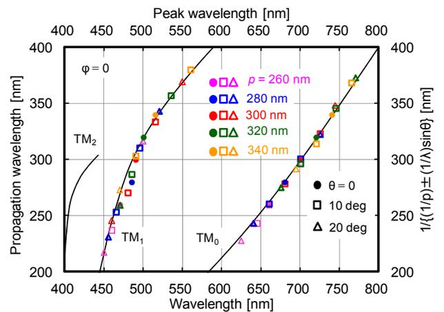
Fig. 5 Comparison between relationships of the calculated propagation wavelengths of the SOI waveguide modes vs. free-space wavelength (lower and left axes) [3], and the experimental peak wavelengths of the external QE vs. corresponding lateral wavelength of forward and backward waves (upper and right axes) for the case of  $\theta$  variation ( $\phi = 0$ ).
