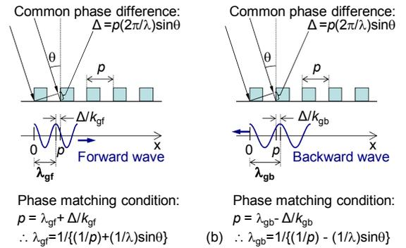
Fig. 4 Schematic diagrams of phase matching conditions between diffracted lights and (a) forward and (b) backward waves in the SOI waveguide.  $\lambda_{\text{gf}}$  and  $\lambda_{\text{gb}}$  are wavelengths of the forward and backward waves, respectively.  $k_{\text{gf}} = 2\pi / \lambda_{\text{gf}}$  and  $k_{\text{gb}} = 2\pi / \lambda_{\text{gb}}$  are wavenumbers for forward and backward waves, respectively.
