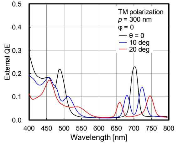
Fig. 3 Measured spectroscopic external quantum efficiencies (QEs) for different incident angle  $\theta$  ( $\phi = 0$ ) with TM-polarized light and Ag L/S grating period  $p = 300 \text{ nm}$ .
