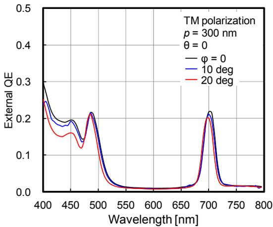
Fig. 2 Measured spectroscopic external quantum efficiencies (QEs) for different incident angle  $\phi$  ( $\theta = 0$ ) with TM-polarized light and Ag L/S grating period  $p = 300 \text{ nm}$ .
