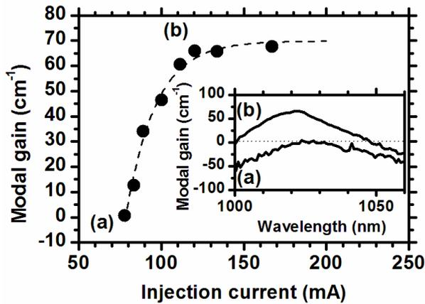
Fig. 3 Maximum modal gain vs injection current. Inset: gain spectra operated at (a) 68.6 mA and (b) 107.2 mA.
