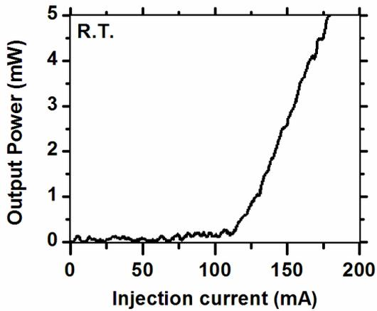
Fig. 1 Output power vs injection current of the device.
