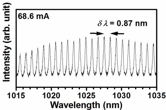
Fig. 2 Amplified spontaneous emission (ASE) spectra obtained at injection current of 68.6mA.
