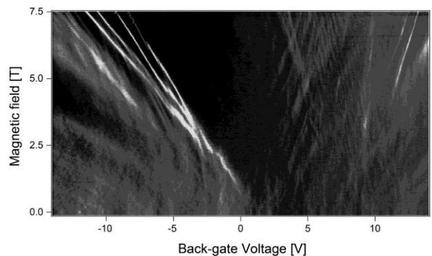
Fig.2. A gray scale plot of the current (for  $V_{sd} = 500$   $\mu$ V) as a function of  $V_g$  and  $B$  at  $T = 0.23$  K. White and black regions correspond to a current of less than 15 pA and more than 40 pA, respectively.
