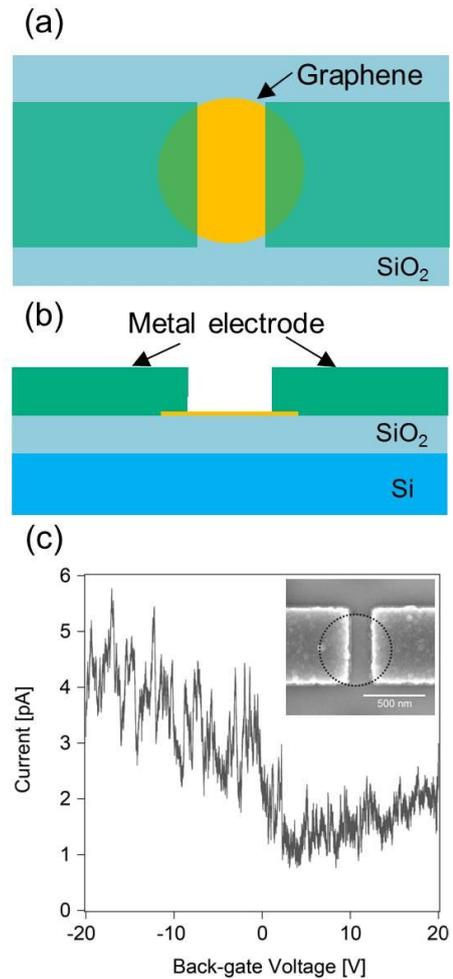
Fig.1. (a) Schematic picture of a designed graphene device. (b) A side-view schematic of the device. (c) Current through the device as a function of  $V_g$  at  $V_{sd} = 100$   $\mu$ V,  $B = 0$  T and  $T = 1.7$  K. Inset. A scanning electron microscopic image of the measured device. The patterned graphene mesoscopic structure is in the dashed-black circle.
