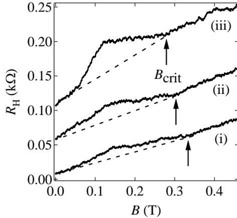
Fig. 2: Hall resistance  $R_H$  as a function of magnetic field  $B$  for various back-gate voltage  $V_{BG}$  at temperature  $T = 10$  K. Back-gate bias voltage was  $V_{BG} =$  (i) -50 V, (ii) -41 V, and (iii) -32 V, respectively (Dirac point is located at  $V_{BG} = -0.6$  V). The  $R_H$  curves are offset vertically by 0.05 k $\Omega$  for clarity.
