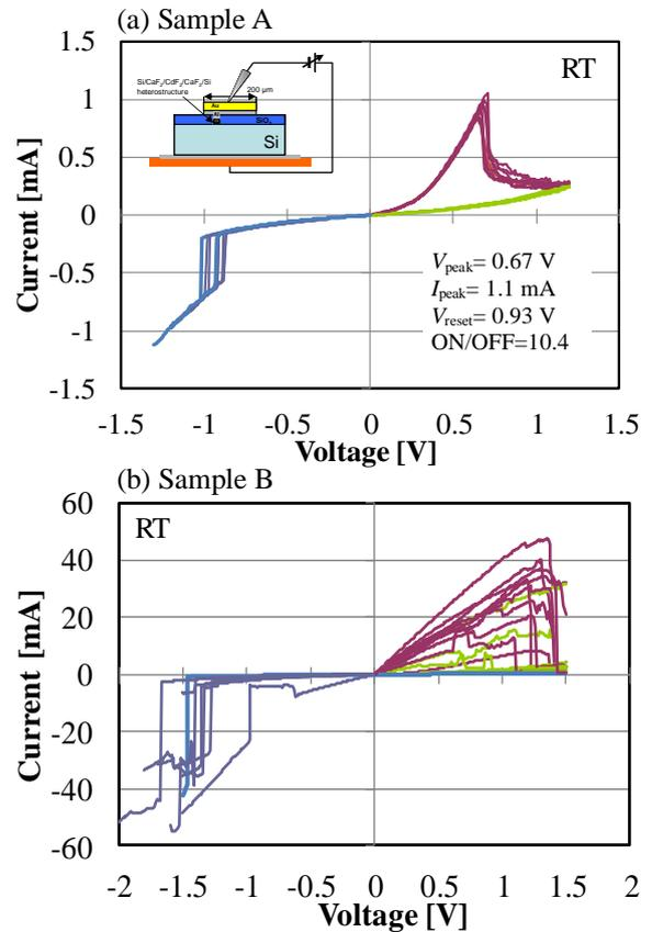
Fig. 3 I-V curve at room temperature exhibiting bipolar resistance switching operation for cyclic set/reset bias sweep. (a) for sample A (with thin oxide during the silicidation) and (b) for sample B (w/o thin oxide).
