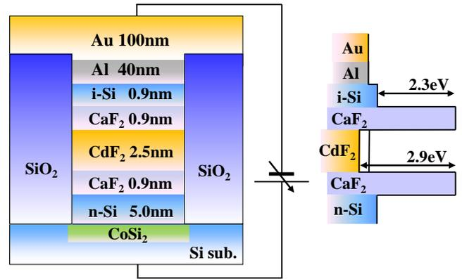
Fig. 1 Schematic device structure and conduction band profile.
