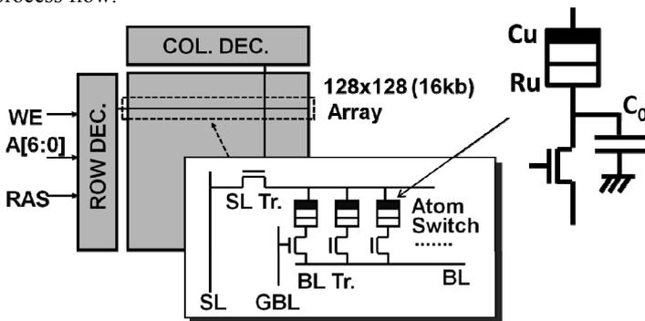
Figure 3. Measurement configuration of atom switch connected to two transistors: BL Tr. and SL Tr. in 16kb switch array. BL Tr. controls SET current. Node between atom switch and BL transistor is loaded by parasitic capacitance of 44 or 0.56fF (=C<sub>0</sub>).
