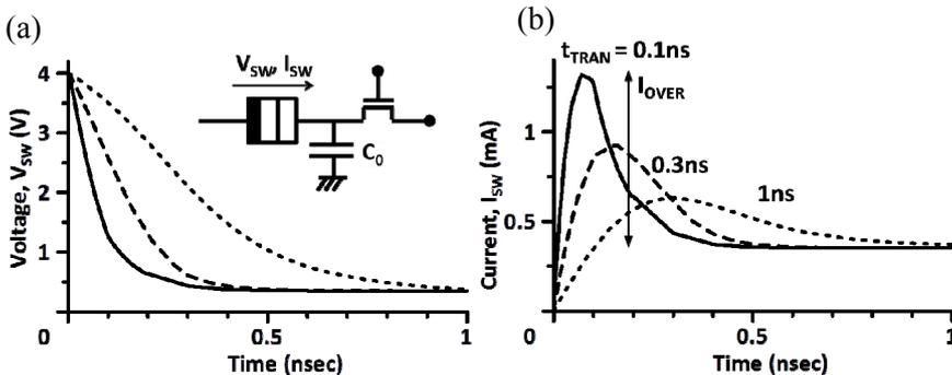
Figure 7. Calculated (a) transient voltage ( $V_{SW}$ ) and (b) current ( $I_{SW}$ ) of atom switch during SET operation with  $C_0=44\text{fF}$  and  $V_{SL}=4\text{V}$ . Resistance of atom switch is linearly changed within  $t_{TRAN}$ .
