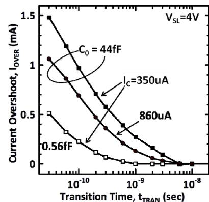
Figure 8. Current overshoot ( $I_{OVER}$ ) in Fig.7. Current overshoot for different condition is also calculated.
