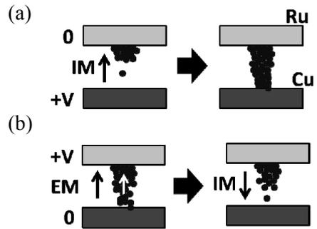
Figure 2 Schematic of (a) SET and (b) RESET operation.
