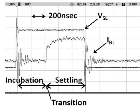
Figure 4. Current on BL ( $I_{BL}$ ) during SET operation for pulse voltage on SL ( $V_{SL}$ ). SET process composed of 3 steps: "Incubation", "Transition", and "Settling" steps.
