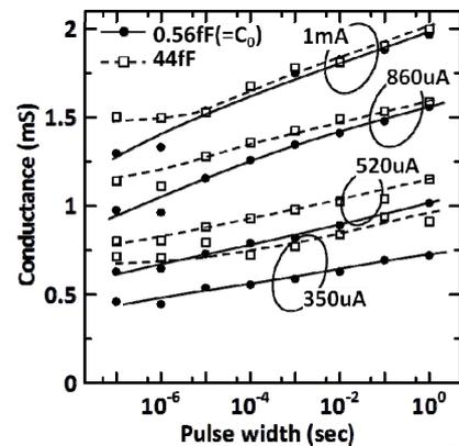
Fig. 6 Conductance at one sigma in Fig.5 for different voltage pulse-width or control current I<sub>C</sub>.
