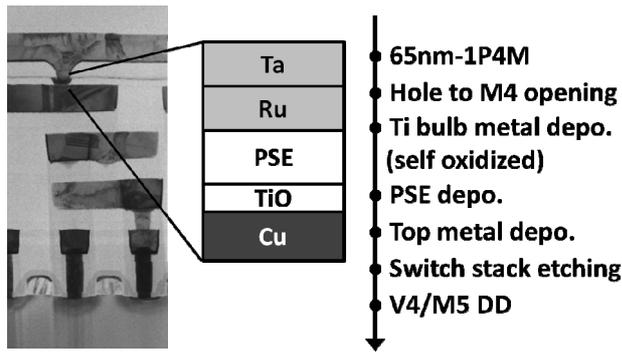
Figure 1. TEM image of atom switch embedded in 65nm 1P5M CMOS, schematic atom-switch stack using PSE/TiO<sub>2</sub> solid electrolyte and process flow.
