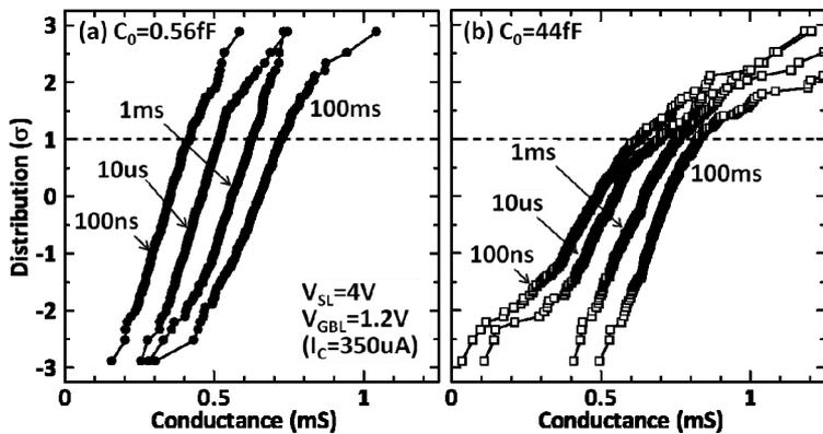
Figure 5. Distribution of ON conductance for different parasitic capacitance of (a) 0.56fF and (b) 44fF and different pulse width. Current is controlled at 350uA (=I<sub>C</sub>) by BL transistor.
