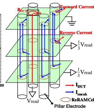
**Fig.11** The schematic of the read operation for a (2\*2\*3) 3D array. The possible sneak leakage paths during read operation are shown.
