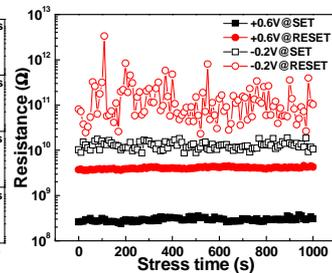
**Fig.14** Read disturbance test. Both RESET and SET states show negligible read disturbance under both read voltages for 1,000s.
