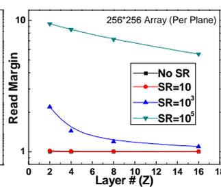
**Fig.15** Read margin calculation for a 256\*256 tile per plane for various layer numbers. SR = 10<sup>5</sup> is needed for 1Mb tile size.
