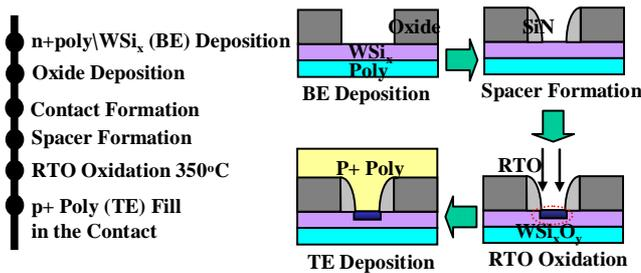
**Fig.1** Key process flow for p+ Poly/WSi<sub>x</sub>O<sub>y</sub> ReRAM device. The memory area is self aligned after contact hole formation. 350°C RTO is used to convert the WSi<sub>x</sub> into WSi<sub>x</sub>O<sub>y</sub>. Finally, p+ Poly is deposited above the WSi<sub>x</sub>O<sub>y</sub> as the top electrode.
