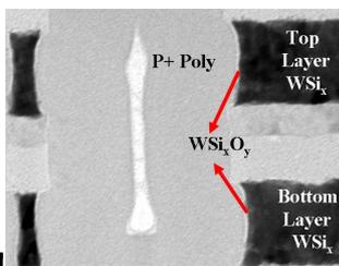
**Fig.9** TEM picture for the 2-layer sidewall WSi<sub>x</sub>O<sub>y</sub> device. The thickness of oxidation for both bottom and top layers is 40Å.
