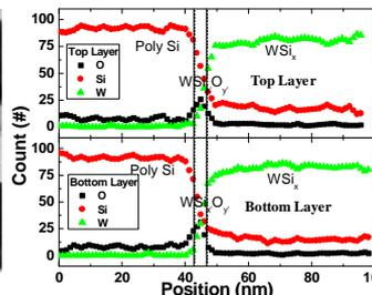
**Fig.10** EDX analysis for the 2-layer WSi<sub>x</sub>O<sub>y</sub> device. The thickness of oxidation for both bottom and top layers is 40Å.
