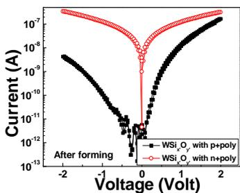
**Fig.4** After forward forming voltage (negative for n+ poly/WSi<sub>x</sub>O<sub>y</sub> and positive for p+ poly/WSi<sub>x</sub>O<sub>y</sub>), symmetric I-V is obtained for n+ poly/WSi<sub>x</sub>O<sub>y</sub>, but asymmetric I-V is obtained for p+ poly/WSi<sub>x</sub>O<sub>y</sub>.
