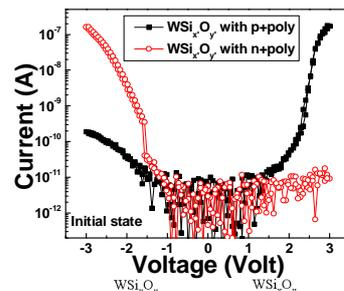
**Fig.3** I-V curves and band diagrams for p+ poly/WSi<sub>x</sub>O<sub>y</sub> and n+ poly/WSi<sub>x</sub>O<sub>y</sub>, respectively. Negative voltage is forward bias for n+ poly, and reverse bias for p+ poly.
