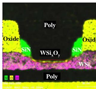
**Fig.2** EDX mapping for the self rectifying poly/WSi<sub>x</sub>O<sub>y</sub> cell. The WSi<sub>x</sub>O<sub>y</sub> is also formed by 350°C RTO and is about 40Å. Then the poly film is deposited as the top electrode.
