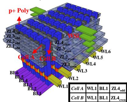
**Fig.8** Proposed 3D structure for WSi<sub>x</sub>O<sub>y</sub> based ReRAM and operation table. The pillar electrode is p+ poly while the sidewall ReRAM is WSi<sub>x</sub>O<sub>y</sub>. WL and BL are used to select the transistor which defines the X-Y coordinate of the pillar electrode. ZL is used to define Z coordinate. Each cell contains two devices.
