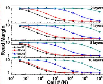
**Fig.13** Read margin calculation with fixed resistance window of 10X (HRS/LRS) for various vertical layers. The self-rectification (SR) is a critical parameter that determines the feasible array size.
