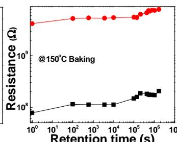
**Fig.7** Retention test at 150°C of the self-rectifying p+ poly/WSi<sub>x</sub>O<sub>y</sub> ReRAM cell. The resistance window is well maintained after 470 hours of baking.
