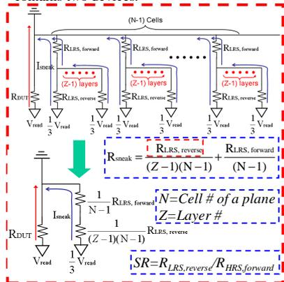
**Fig.12** Worst-case read margin. The adjacent cells near the selected cell are all in LRS.
