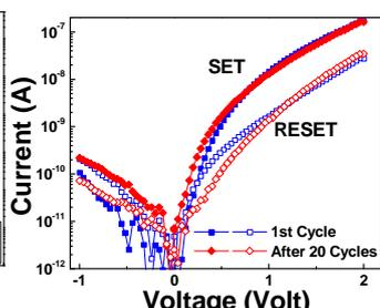
**Fig.5** Read I-V curves for RESET and SET. The self-rectifying property is well preserved after cycling. Both RESET and SET show low leakage current under reverse bias.
