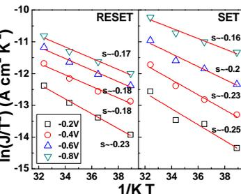
**Fig.6**  $\ln(J/T^2)$  versus  $1/k_B T$  curves for the RESET and the SET states at various biasing voltages. The behaviors are well predicted by thermionic emission.
