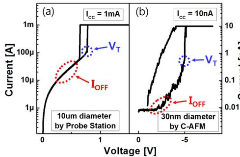
Fig. 4 TS characteristic of  $NbO_x$  selector device measured (a) by probe station and (b) by C-AFM.
