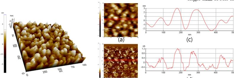
Fig. 6 Surface morphology of  $NbO_x$  selector device.
