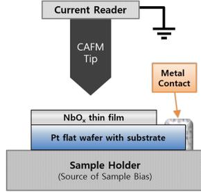
Fig. 2 Schematic diagram of C-AFM measurement.
