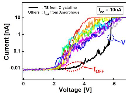
Fig. 5 Various I-V curves from local spots ( $\sim 30\text{nm}$  size) with two trends. One is TS behavior with low  $I_{OFF}$  from crystalline phase and the other is tunneling current with high  $I_{leak}$  from amorphous phase.
