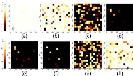
Fig. 9 Response of local spots under gradually changing bias. Each rectangular area represents a local spot. (a) 3V, (b) 5V, (c) 7V, (d) 8V while increasing bias, and (e) 8V, (f) 7V, (g) 5V, (h) 3V while decreasing bias. Several spots showed TS under 3V while some other spots showed leakage current at same bias.
