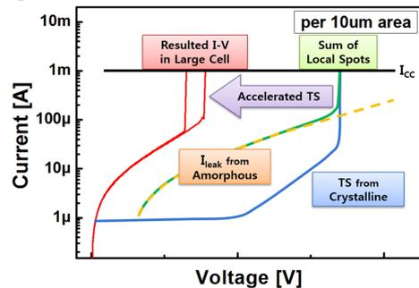
Fig. 10 Explanation for the difference in I-V curves 4(a) and (b). With the transferred heat induced TS acceleration effect, sum of all currents from local spots will be same as I-V from larger cell. Scales are normalized.
