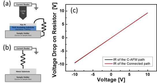
Fig. 3 Schematic diagrams of confirming reliability (a) by C-AFM path and (b) by connected path. (c) I-V curves of a typical resistor from (a) and (b).
