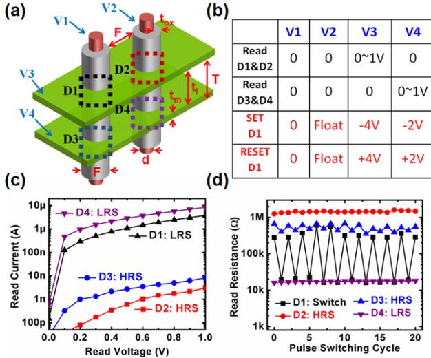
Fig. 3 (a) A schematic of  $2 \times 2$  3D cross-point array. (b) Summary of operation voltages for read/write schemes (c) Measured readout current for the cells after the read operation applied. (d) Measured resistances when D1 is switched repeatedly, while the states of other cells remain unchanged.
