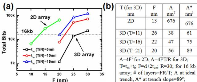
Fig. 4 (a) The relation between the max total bits for an array (2D as well as 3D) and the half-pitch  $F$  for different  $t_m$ . To achieve 16k total bits, min  $F$  can be estimated at  $F = 13$  nm in 2D. (b) The integration density (cell area per bit).
