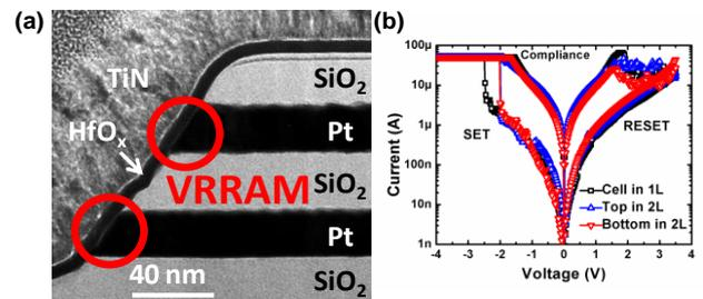
Fig. 2 (a) TEM of the double-layer (2L)  $\text{HfO}_x$ -based vertical RRAM. The  $\text{HfO}_x$  thickness is 5nm. (b) Typical DC I-V switching characteristics.
