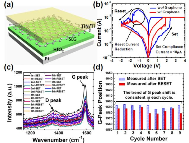
Fig. 5 (a) SLG is inserted between the top electrode and metal oxide layer. (b) Typical I-V curves of Graphene-RRAM and control sample. Significant reduction of RESET current is observed (c) 9 cycles of Raman data measured after SET and RESET cycles at the same location. (d) The position of G peak as a function of switching cycle: consistent shift over 9 switching cycles.
