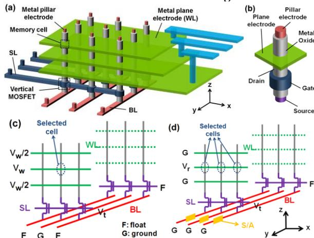
Fig. 1 (a) Schematic of a 3D vertical RRAM cross-point array. (b) The details of the structure: the switching metal oxide material is sandwiched between the plane electrode and the vertical pillar electrode. (c) and (d) show the write and read bias conditions, respectively.
