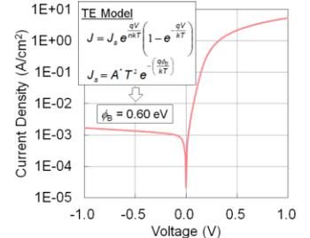
**Fig. 4** J-V characteristics of the NiGe/n-Ge without implant. Based on thermionic emission (TE) model with ideality factor ( $n$ ), the SBH ( $\phi_b$ ) of NiGe/n-Ge is found to be 0.60 eV.
