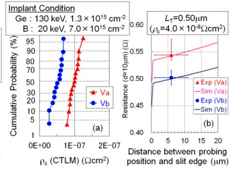
**Fig. 9** (a)  $\rho_c$  values measured by CTLM depend on the position of voltmeters. (b) 2-D DC simulation results by changing  $L_T$  as a fitting parameter. The extracted  $\rho_c$  was  $4.0 \times 10^{-8} \Omega \text{ cm}^2$ . Activation was performed at  $540^\circ \text{C}$  for 10 sec. Ni thickness was 20 nm.
