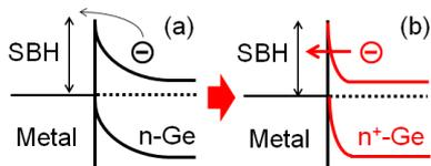
**Fig. 1** Illustration of a concept in this work to acquire low  $\rho_c$  by the CAE techniques. Band diagrams for metal/n-Ge contacts are shown, for example, indicating (a) high  $\rho_c$  with low carrier concentration and (b) low  $\rho_c$  with high carrier concentration due to a thin thickness of a tunneling region.
