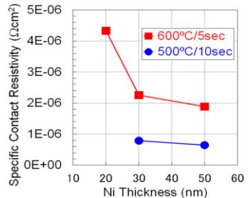
**Fig. 6**  $\rho_c$  values for the NiGe/ $n^+$ -Ge contact samples. The P/Sb co-implant condition was the same as Fig. 5(a). The lowest  $\rho_c$  value was  $6.4 \times 10^{-7} \Omega \text{ cm}^2$ .
