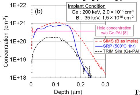
**Fig. 5** Concentration profiles for (a)  $n^+$ -Ge and (b)  $p^+$ -Ge by applying the CAE techniques. A maximum electron concentration of  $8.6 \times 10^{19} \text{ cm}^{-3}$  and a world record hole concentration of  $8.4 \times 10^{20} \text{ cm}^{-3}$  have been confirmed. These values are higher than those for single P implant and B implant without Ge-PAI, respectively.
