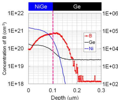
**Fig. 10** SIMS profile of the NiGe/ $p^+$ -Ge contact sample for the  $\rho_c$  of  $4.0 \times 10^{-8} \Omega \text{ cm}^2$ . The boron concentration at the NiGe/ $p^+$ -Ge interface is  $7 \times 10^{20} \text{ cm}^{-3}$ .
