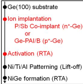
**Fig. 2** A process flow with just one mask step for obtaining low  $\rho_c$  samples.
