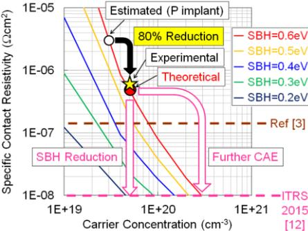
**Fig. 8** Theoretical calculation of  $\rho_c$  on n-Ge(100) showing excellent consistency with the experimental  $\rho_c$ . The CAE technique is considered to have reduced  $\rho_c$  by 80%. The obtained  $\rho_c$  using NiGe is slightly higher than the best value ever reported for n-Ge using different contact materials with the lower SBH [3]. To achieve the  $\rho_c$  for ITRS 2015 for NMOS, further CAE improvement and/or SBH reduction is required.
