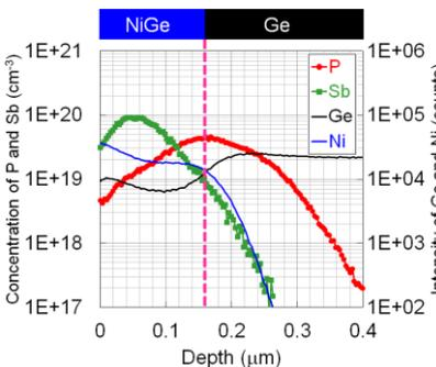
**Fig. 7** SIMS profile of the NiGe/ $n^+$ -Ge contact sample for the  $\rho_c$  of  $6.4 \times 10^{-7} \Omega \text{ cm}^2$ . The dopant concentration at the NiGe/ $n^+$ -Ge interface is  $5 \times 10^{19} \text{ cm}^{-3}$ . Ge and Ni signals are used to determine the NiGe/ $n^+$ -Ge interface.
