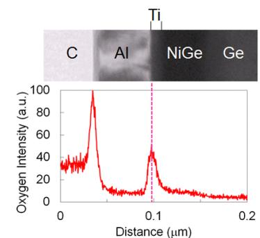
**Fig. 12** TEM image and the oxygen intensity (EDX) of the NiGe/ $p^+$ -Ge contact sample. An oxide layer between Al and Ti films was confirmed. We think this oxide layer induces the higher  $\rho_c$  value than the theoretical one.
