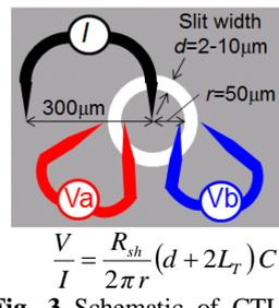
**Fig. 3** Schematic of CTLM for evaluating  $\rho_c$ . The resistance of each contact sample was measured twice with changing probing positions.
