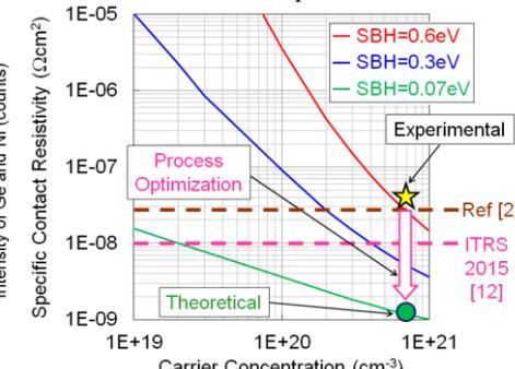
**Fig. 11** Theoretical calculation of  $\rho_c$  on p-Ge(100) and the experimentally obtained  $\rho_c$ . The process optimization will achieve the theoretical  $\rho_c$  of  $1 \times 10^{-9} \Omega \text{ cm}^2$  for PMOS.
