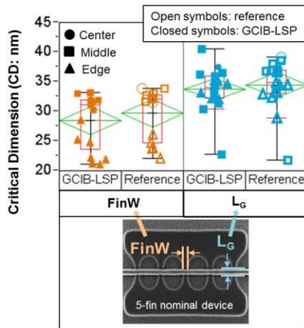
Fig.3 Inline CD data of finW and gate length (L<sub>G</sub>).
