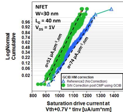
Fig.6: Saturation drive current\**t*<sub>inv</sub> at offset V<sub>TH</sub> with (closed symbols) and without (open symbols) GCIB-LSP correction on short channel transistors. FinW=30nm, L<sub>G</sub>=40 nm, V<sub>DS</sub>=1V.
