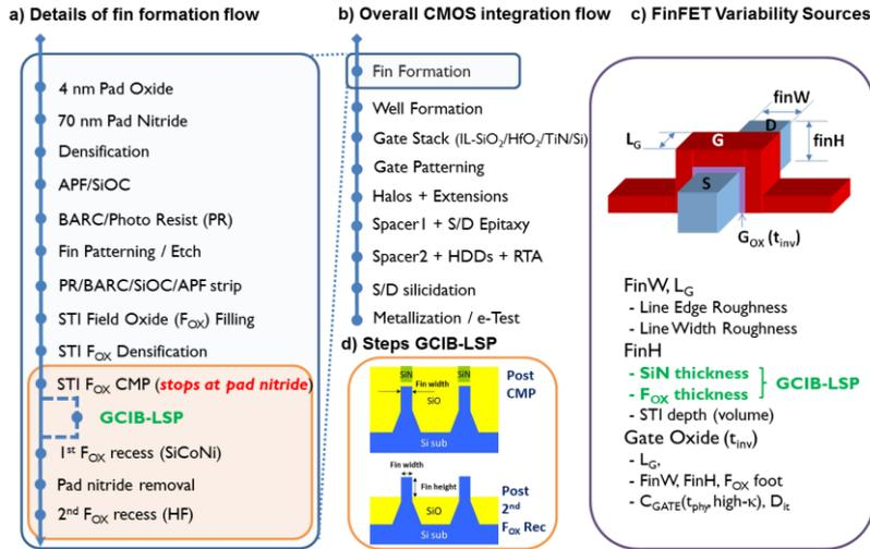
Fig. 1 Process flow of bulk finFET device fabrication (a, b), sources of inline process variation (c), and process step where GCIB was applied to reduce finH variation (d).
