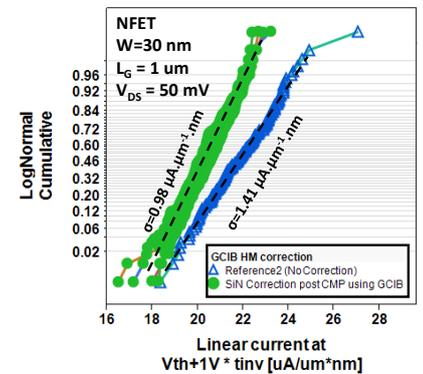
Fig.5 Linear drive current\**t*<sub>inv</sub> at offset V<sub>TH</sub> with (closed symbols) and without (open symbols) GCIB-LSP correction. FinW=30nm, L<sub>G</sub>=1 μm.
