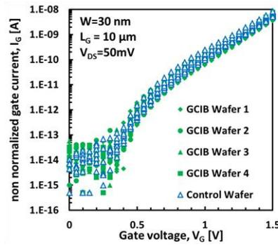
Fig. 4 Gate current I<sub>G</sub> vs. gate voltage V<sub>G</sub> for bFF with (closed symbols) and without (open symbols) GCIB-LSP correction. FinW=30nm, L<sub>G</sub>=10 μm.
