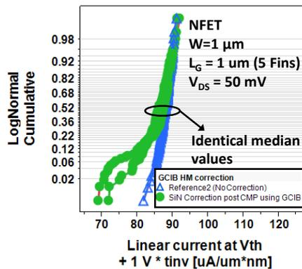
Fig. 7: Linear drive current\**t*<sub>inv</sub> at offset V<sub>TH</sub> with (closed symbols) and without (open symbols) GCIB-LSP correction. finW=1μm, L<sub>G</sub>=1 μm.
