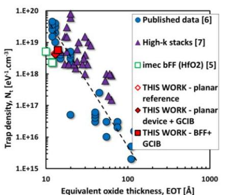
Fig. 8: Trap density extracted from Low Frequency Noise spectral density vs. EOT.
