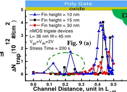
**Fig. 9** (a)  $\Delta N_{trap}$  profiling for different Fin-height trigate devices after HC stress. More traps are observed for lower Fin-height device as a result of larger electric field. (b) The illustration of the high electric field at the low fin height device which will induce larger electric field in devices under HC stress.
