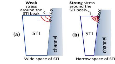
**Fig. 13** (a) The illustration of a wide STI; (b) the illustration of a narrow STI. The narrower the STI is, the stronger the field is around the corner between STI and channel.
