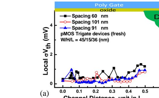
**Fig. 12** (a) The different fin spacing affects the variation of fresh devices. (b) To study the Fin spacing effect on the degradation of stressed trigate devices, three different spacing devices were measured.
