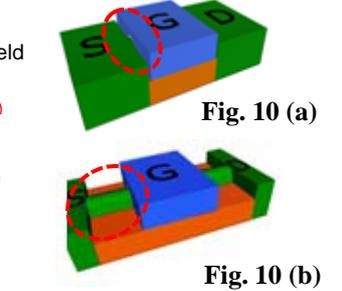
**Fig. 10** The illustration of two different bulk trigate devices with (a) low  $R_{sd}$  (the covered Fin), (b) high  $R_{sd}$  (the uncovered Fin).
