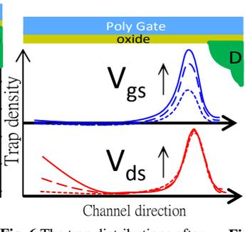
**Fig. 6** The trap distributions after different HC stress schemes. For increase of  $V_{gs}$ , the peak near drain side grows. For increase of  $V_{ds}$ , the region near channel middle grows.
