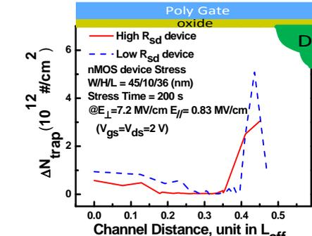
**Fig. 11** The trap densities profiled along the transverse direction of channel. Since the electric field in the channel can be reduced by the exterior S/D resistance on the fin, it was found that the trap density after HC stress for high  $R_{sd}$  shows a low degradation than that for lower  $R_{sd}$ .
