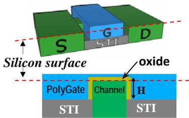
**Fig. 1** (top) The 3D structure of bulk trigate devices with poly/SION in the channel cause the variation of the threshold voltage; (bottom) the cross-sectional view of bulk trigate devices with fin height H.
