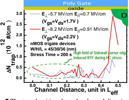
**Fig. 7** The trap densities along the channel direction after strong or weak HC stress. It was found that the peaks are not only near the drain edge but also in the channel region after HC stress, and the stronger the HC stress is, the higher they become.
