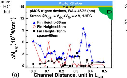
**Fig. 14** (a)  $\Delta N_{trap}$  profiling for different Fin-height trigate devices after NBTI stress. More traps are observed for larger Fin-height device as a result of sidewall roughness effect. (b) Interface trap density of Fin structure was measured by different fin-heights devices. The amount of interface traps contributed by the fin-width only can be obtained from the plot by extrapolating the measured data to zero fin-height.
