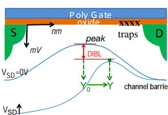
**Fig. 3** The traps detected by the channel barrier peak will dominate the  $V_{th}$  variation for the device after the stress. By varying the  $V_{sd}$ , the barrier peak will be shifted toward the drain such that the trap density can be profiled along the channel.
