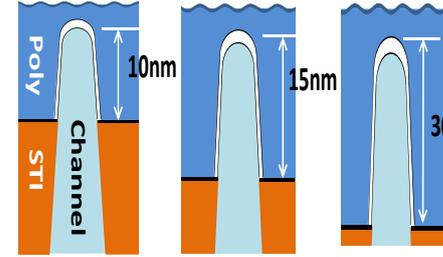
**Fig. 8** To study the impacts of the sidewall on the degradation of stressed trigate devices, three different sidewall devices were prepared.
