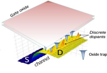
**Fig. 2** For fresh devices, the discrete dopants in the channel cause the variation of the threshold voltage. For stressed devices, the interface-trap induced trap barriers will also give rise to the threshold voltage variation.
