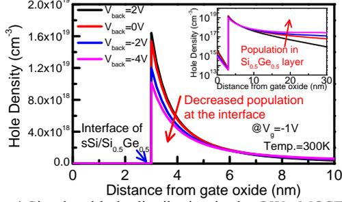
Fig. 4 Simulated hole distribution in the QW pMOSFET when  $V_g = -1V$  at 300K under various back-gate biases through Medici.
