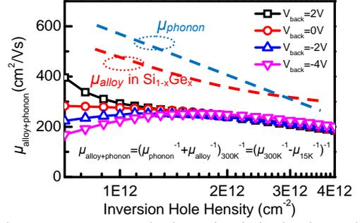
Fig. 6  $\mu_{\text{alloy+phonon}}$  versus the inversion hole density under different back-gate biases obtained from the measured hole mobility at 300K and 15K.
