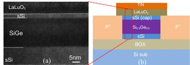
Fig. 1 (a)TEM images of the sSi/Si<sub>0.5</sub>Ge<sub>0.5</sub>/sSOI substrate after S/D annealing; (b)Schematic view of the sSi/Si<sub>0.5</sub>Ge<sub>0.5</sub>/sSOI QW pMOSFET with LaLuO<sub>3</sub> as gate stacks.
