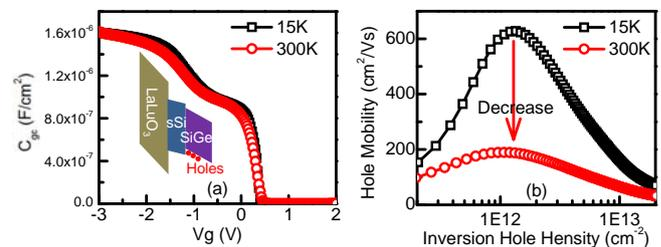
Fig. 2 (a) Measured split C-V characteristics of QW pMOSFET at 15K and 300K after correction of the overlap capacitance; (b) Measured Hole mobility of the QW pMOSFETs at 15K and 300K.
