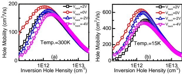
Fig. 5 Measured hole mobility of the QW pMOSFET under various back-gate biases at (a) 300K and (b) 15K.
