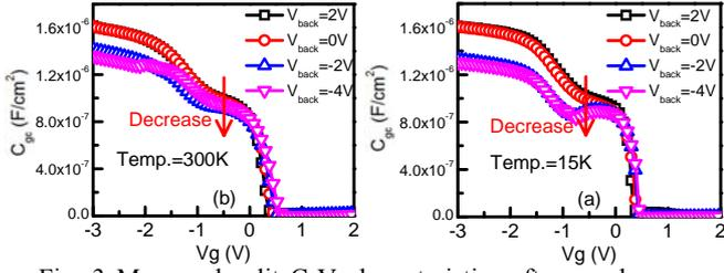
Fig. 3 Measured split C-V characteristics after overlap capacitance correction of QW pMOSFET under various back-gate biases at (a) 300K and (b) 15K.
