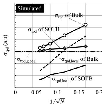
Fig. 8 Simulated  $\sigma_{\tau_{pd}}$  -  $1/\sqrt{N}$  relationship.  $\sigma_{\tau_{pd,local}}$  and  $\sigma_{\tau_{pd,global}}$  denote local and global variability, respectively.  $\sigma_{\tau_{pd}}$  is defined by root sum square of  $\sigma_{\tau_{pd,local}}$  and  $\sigma_{\tau_{pd,global}}$ .
