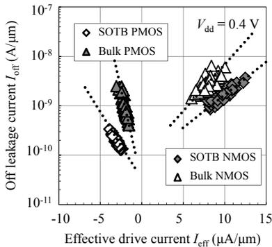
Fig. 4  $I_{eff}$ - $I_{off}$  characteristics for SOTB and bulk. SOTB has higher  $I_{eff}$  than bulk at the same  $I_{off}$ .
