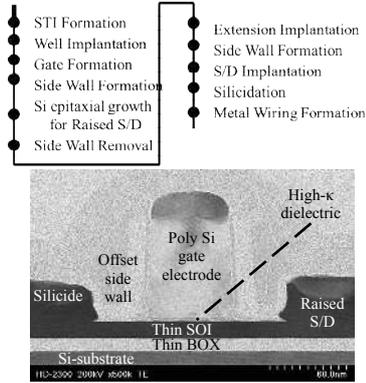
Fig. 1 Fabrication process and TEM image of SOTB transistor.
