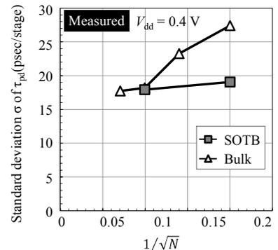
Fig. 6 Measured  $1/\sqrt{N}$  dependence of standard deviation of propagation delay time ( $\sigma_{\tau_{pd}}$ ).
