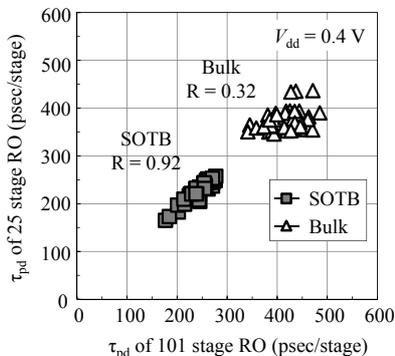
Fig. 7 Correlation between delays of 101- and 25-stage ROs. The correlation coefficients are  $R = 0.92$  and  $0.32$  for SOTB ( $\blacksquare$ ) and bulk ( $\blacktriangle$ ), respectively.
