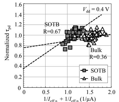
Fig. 9 Relation between normalized  $\tau_{pd}$  ( $\tau_{pd}/\text{median}$ ) and  $1/I_{eff,n} + 1/I_{eff,p}$ .  $I_{eff,n}$  and  $I_{eff,p}$  denote effective drive currents of N and PMOS, respectively.
