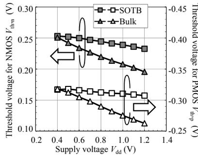
Fig. 2 Supply voltage ( $V_{dd}$ ) dependence of threshold voltage ( $V_{th}$ ).
