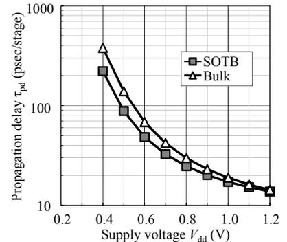
Fig. 3 Supply voltage ( $V_{dd}$ ) dependence of propagation delay time.
