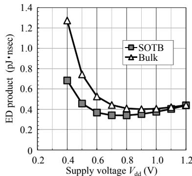
Fig. 5 Supply voltage ( $V_{dd}$ ) dependence of energy-delay product of 101 stage RO. Energy is defined by  $I_{dd}V_{dd}$  / frequency.  $I_{dd}$  is active current of RO.
