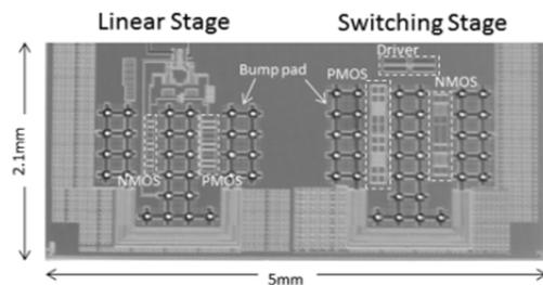
Fig. 6. Fabricated chip photograph of CMOS EA.
