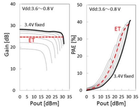
Fig. 3. Measured 1.95GHz CW characteristics. The dotted line shows Gain and PAE when ET with envelope modulation is adopted.
