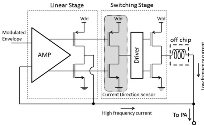
Fig. 2 Schematic of designed CMOS envelope amplifier.
