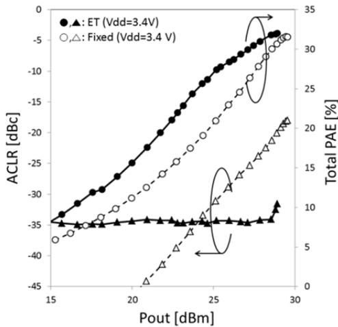
Fig. 4. Comparison of PAE and ACLR in the case where the ET or fixed Vdd is adopted for a W-CDMA signal.
