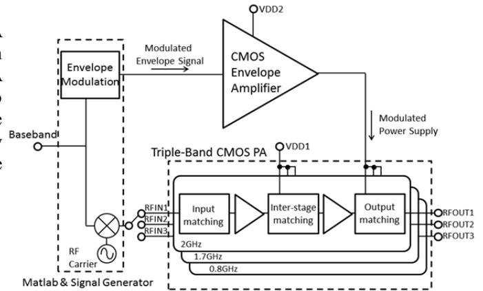
Fig. 1. Block diagram of the envelope tracking power amplifier performance measurement system.
