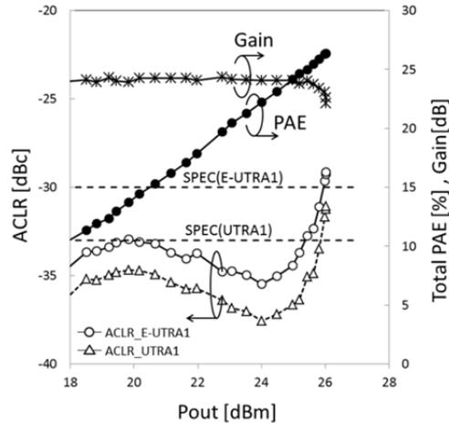
Fig. 5. Measurement results of PAE, Gain and ACLR versus Pout for 10 MHz LTE signal at 1.95 GHz.
