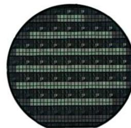
Fig. 2 Photograph of fabricated GaN MIS-HEMTs over 6-inch Si wafer.
