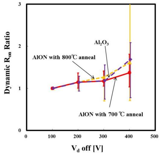
Fig. 4 Measurement results of dynamic  $R_{on}$  ratio versus drain voltage. Dynamic  $R_{on}$  ratio is defined as the dynamic on-resistance at each drain voltage divided by the dynamic on-resistance at drain voltage of 100 V. Error bar was inserted corresponding to the variation across a wafer.
