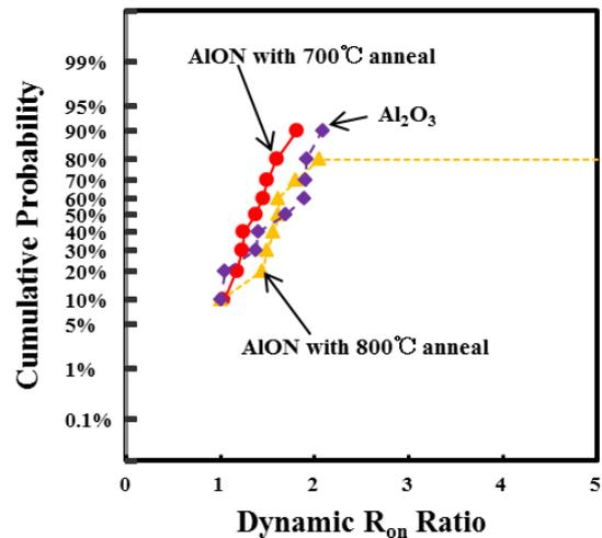
Fig. 5 Cumulative probability distribution of dynamic  $R_{on}$  ratio at  $V_d=400$  V across an all over the 6-inch wafer.
