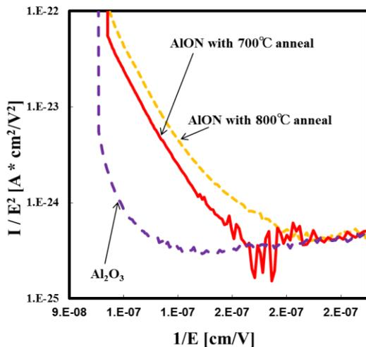
Fig. 3 Data are presented as a FN plot showing the dependence of leakage current divided by electric field squared versus reciprocal electric field. The liner slope implies FN tunneling in insulator.
