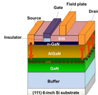
Fig. 1 Schematic cross-sectional view of normally-on type Al-GaN/GaN MIS-HEMT structure used in this work.
