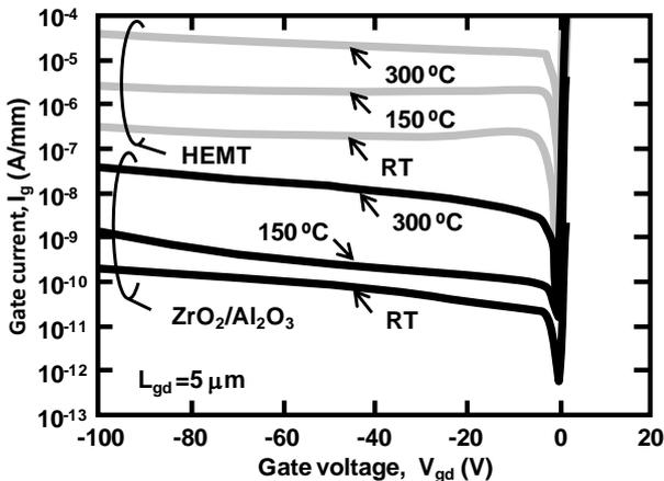
Fig. 4 Gate leakage current for ZrO<sub>2</sub>/Al<sub>2</sub>O<sub>3</sub> MISHEMT and Schottky-gated HEMT.
