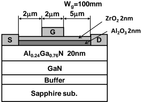
Fig. 1 Schematic cross-sectional structure of ZrO<sub>2</sub>/Al<sub>2</sub>O<sub>3</sub> MISHEMT.
