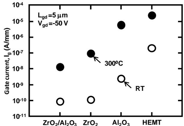
Fig. 5 Gate leakage current for all devices at RT and 300 °C.
