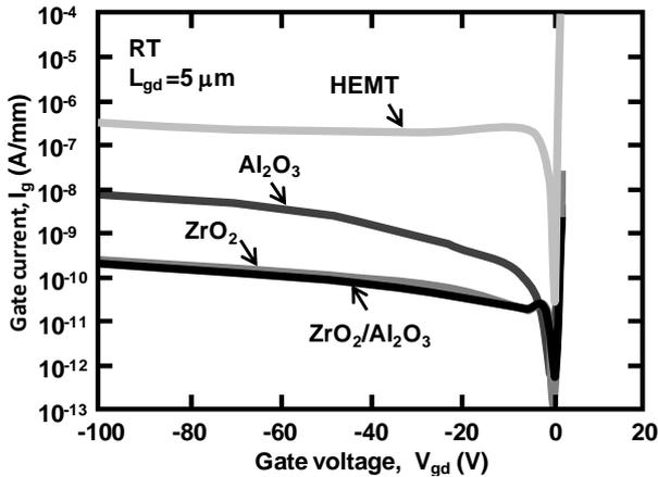
Fig. 3 Two-terminal gate-drain leakage current.
