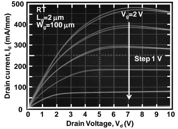
Fig. 2 Id-Vd characteristics for ZrO<sub>2</sub>/Al<sub>2</sub>O<sub>3</sub> MISHEMT measured at RT.
