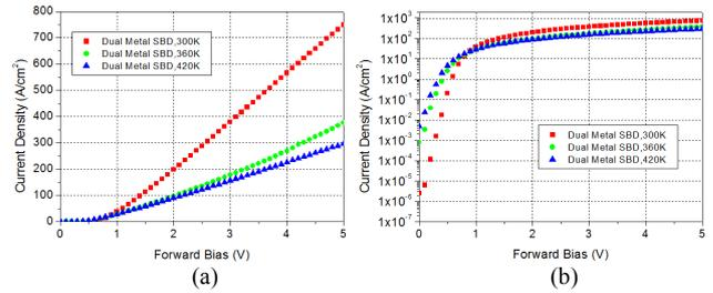
Fig. 5 Temperature dependent analysis of the dual metal SBD in forward characteristics. (a) linear scale (b) semi-log scale
