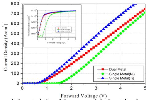
Fig. 2 Forward characteristics of the proposed dual metal and conventional single metal Ni and Ti SBD. The length of Lac is 12  $\mu\text{m}$ .
