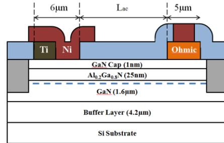
Fig. 1 Cross-sectional schematic of an AlGaIn/GaN dual metal SBD. The width of the device is  $140 \mu\text{m}$ .
