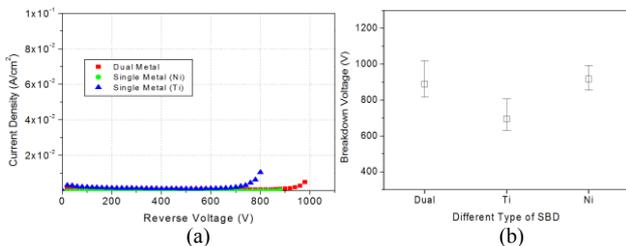
Fig. 4 (a) Breakdown characteristics of the proposed dual metal and single metal Ni and Ti SBDs. (b) Statistics of breakdown voltage obtained from 5 devices in different dies. (Lac = 12  $\mu\text{m}$ )
