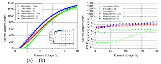
Fig. 6 Comparison between simulation and measurement results of the dual metal SBD and single metal SBDs. (a) forward characteristics. (b) reverse characteristics.
