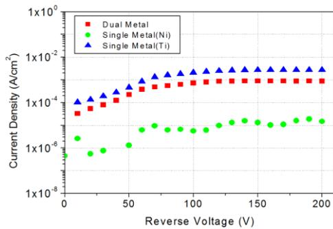
Fig. 3 Reverse characteristics of the proposed dual metal and conventional single metal Ni and Ti SBDs. (Lac = 12  $\mu\text{m}$ )
