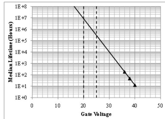
Fig. 4. TDDB results at  $150^\circ\text{C}$  on Generation 2, 1200 V devices. Data points obtained by fitting all lifetime data, including right-censored points. Dashed lines: 20 V and 25 V, for reference.
