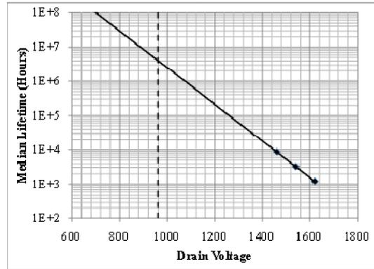
Fig. 3. ALT-HTRB results at  $150^\circ\text{C}$  on Generation 2, 1200 V devices. Data points obtained by fitting all lifetime data, including right-censored points. Dashed line: 960 V fiducial, for reference.
