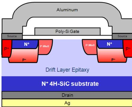
Fig. 1. Schematic cross section of Cree, Inc. vertical DMOSFET Generation 2 device.
