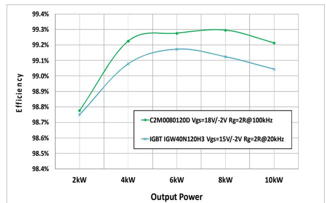
Fig. 5. Comparison of Gen 2 1200 V 80 mΩ SiC MOSFET operating at 100 kHz vs Si IGBT operating at 20 kHz in a 10 kW Boost Converter [2].
