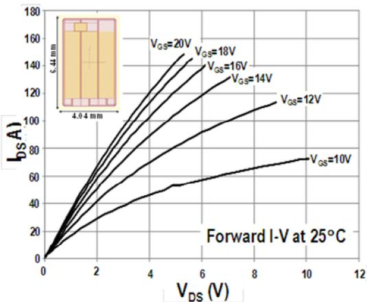
Fig 2. Forward I-V curves for commercial 2<sup>nd</sup> Generation 1200 V, 50 A SiC MOSFET
