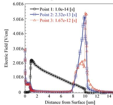
Fig. 5. Electric field distribution along ion track at the times shown in Fig. 4.
