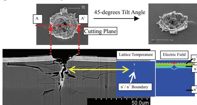
Fig. 1. Cross sectional scanning electron microscope (SEM) view of SEB destruction trace, simulated lattice temperature and electric field at time point 6 shown in Fig. 4.
