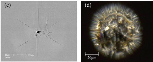
Fig. 3. 3 $\mu\text{m}$  cutting from device surface using FIB: (c) SEM view, and (d) stereomicroscope view.
