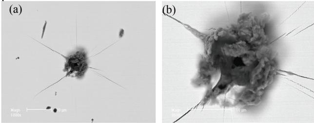
Fig. 2. SEM views of device surface after aluminum etching: (a) overall view and (b) magnified view.
