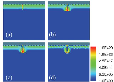
Fig. 6. Impact ionization rate ( $\text{s}^{-1}\text{cm}^{-3}$ ) at the times shown in Fig. 4: (a) point 1, (b) point 3, (c) point 4, and (d) point 5.
