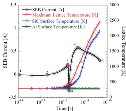
Fig. 4 Simulated SEB current (A) and temperature (K)
