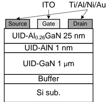
Fig. 1. Cross-sections of the transparent gate AlGaN/GaN HEMT on Si substrate.
