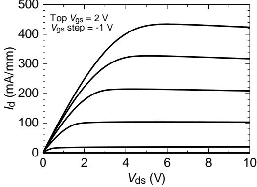
Fig. 3. Typical drain  $I$ - $V$  characteristics of the transparent gate HEMT with a gate length of 3  $\mu$ m.
