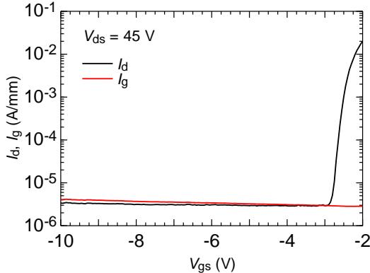
Fig. 4. Drain and gate current as a function of gate voltage for the transparent gate HEMT.
