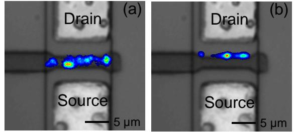
Fig. 5. False color image reporting the distribution of EL of the transparent gate AlGaN/GaN HEMT. Image were taken when the device was continuously stressed at  $V_{ds} = 45$  V and (a)  $V_{gs} = -10$  V (off-state condition), (b)  $V_{gs} = -2$  V (on-state condition).
