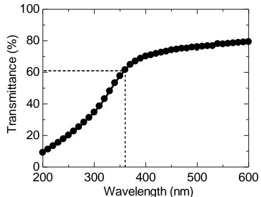
Fig. 2. Transmittance of ITO film as a function of wavelength.
