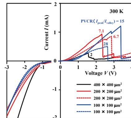
Fig. 2. I-V characteristics for various sized GaN/AlN RTDs.
