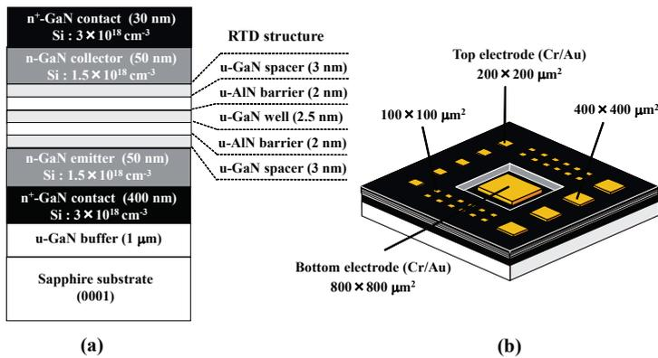
Fig. 1. GaN/AlN RTD grown by MOPVE. (a) Grown and (b) device structures.
