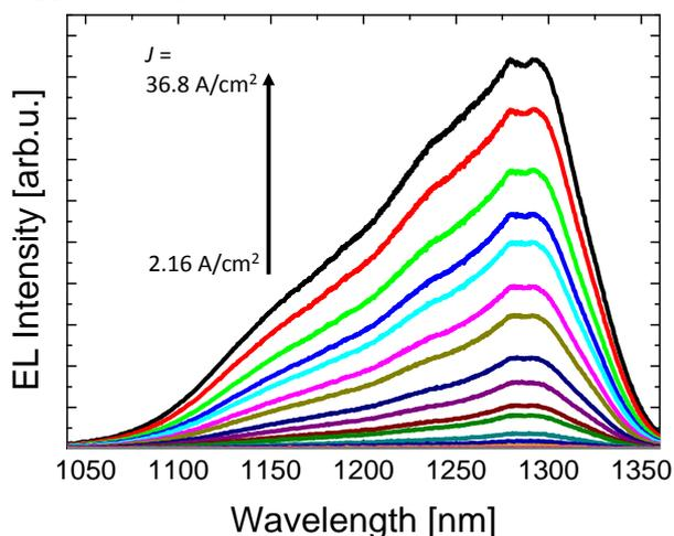
Fig. 2 EL spectra from the RWG including 4-stacked multi-color InAs-QDs with different injection current densities.
