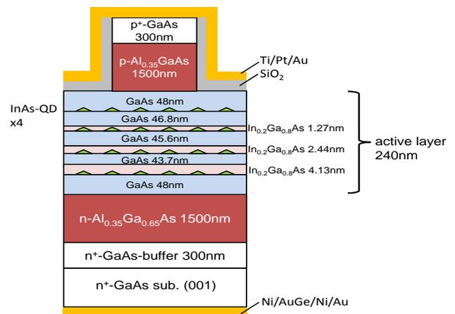
Fig. 1 Schematic profile of a RWG fabricated on a grown sample.
