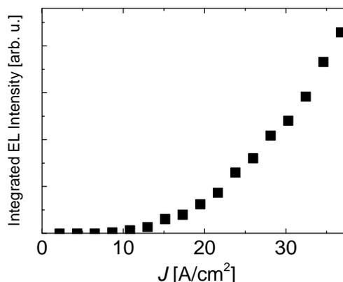
Fig. 3 Integrated EL intensities against injected current densities.
