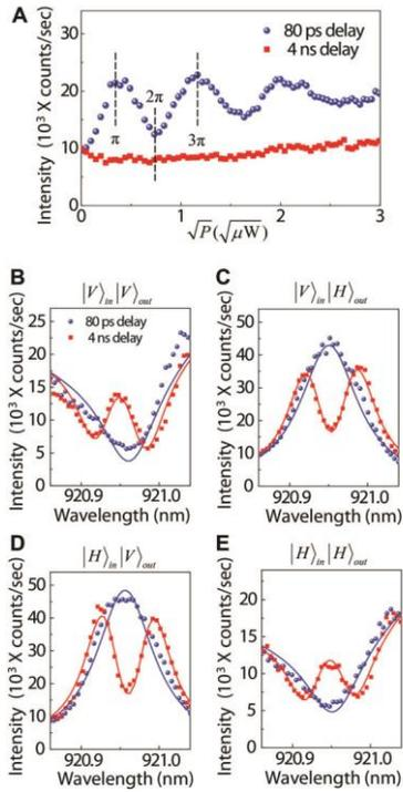
**Figure 2. Demonstration of controlled bit flip by pulsed pump-probe excitation.** (A) Blue circles (red curve) plot the change in the probe signal at 80 ps (4 ns) pump-probe delay time. (B)-(E) CNOT operation for all four combinations of input-output polarizations. Cavity spectra are measured with a  $\pi$  pump pulse.
