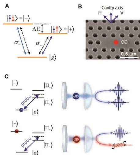
**Figure 1. Implementation of a QD-photon CNOT operation. (A) Energy level structure of a neutral QD coupled to an optical cavity under a magnetic field. (B) SEM image of the fabricated device and the cavity axis relative to the photon polarization. (C) Illustration of CNOT operation.**
