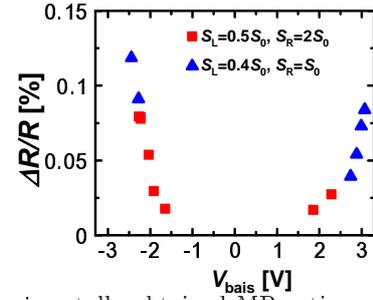
FIG. 3: Experimentally obtained MR ratio as a function of bias voltage between the left and the right electrodes of Fig.2.  $S_0 = 100\mu\text{m}^2$  and  $T=77\text{K}$ .  $V_{\text{bias}} > 0$  corresponds to Fig.2 ( $E_L > 0$ ).  $V_{\text{bias}} < 0$  corresponds to reversed bias direction of Fig.2 ( $E_L < 0$ ).
