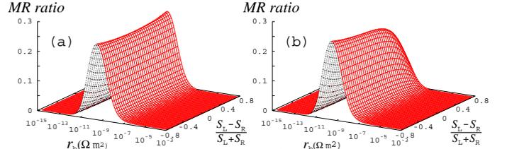
FIG. 4: Calculated MR ratios of the local measurement setup as functions of the interface resistance  $r_b$  and area difference.  $S_L$  and  $S_R$  show areas of the left and right electrodes, respectively. (a) Standard theory (b) Interface electric field is introduced (Eq.(4)).  $\gamma_L = \gamma_R = \beta = 0.10$ .  $t_N=1250\text{nm}$ ,  $l^N=5.1\mu\text{m}$ ,  $r_N = 1.07 \times 10^{-10} \Omega\text{m}^2$ ,  $l^F=5\text{nm}$ ,  $r_F = 4.5 \times 10^{-15} \Omega\text{m}^2$ .
