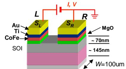
FIG. 2: Schematic diagram of a lateral device. The distance  $t_N$  between the two electrodes is  $t_N = 1\mu\text{m}$ . Thickness of MgO is 1nm.
