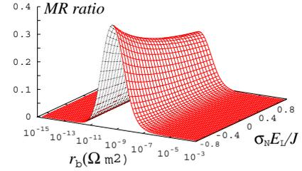
FIG. 5: Calculated MR ratio of the local measurement setup as functions of the left electric field.  $S_L = 4S_R$ . Parameters are the same as Fig.4.
