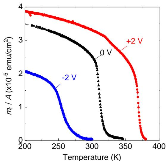
Fig. 1 Temperature dependence of remanent magnetization of Co ultra-thin film under applying gate voltage of +2 V, 0 V, and -2 V.
