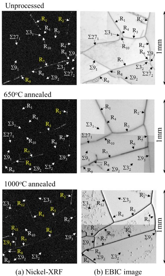
Fig. 1 (a) Nickel signal map in XRF measurement and (b) EBIC image for the same location of XRF maps.
