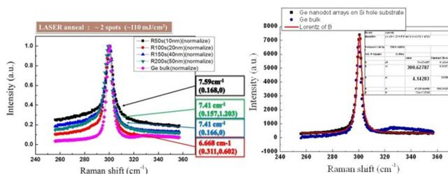
Fig. 2 is show the measurement result of Raman spectrum distribution of the Ge nanodot arrays (a) with different hole depth, (b) the Ge nanodot arrays with moderate hole depth is after laser annealing treatment ( $E = 100\text{ mJ/cm}^2$  of sixteen laser spots).
