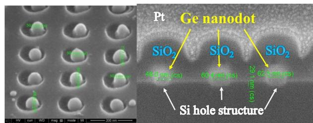
Fig. 3 is showed (a) tilt  $52^\circ$  without the  $\text{SiO}_2$  layer and (b) the cross section SEM images with the  $\text{SiO}_2$  layer of the high quality Ge nanodot arrays, and entire Ge nanodots size is about  $60\text{ nm}$ .
