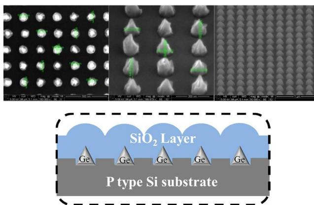
Fig.1 is sho the SEM image of the Ge nanocone arrays (a) top view and (b) tilt  $52^\circ$  is without the  $\text{SiO}_2$  layer, (c) tilt  $52^\circ$  is with the  $\text{SiO}_2$  layer, (d) is schematic cross section of the Ge nanocone arrays (sandwich structure ) All of nanocone arrays are ordered arrangement.
