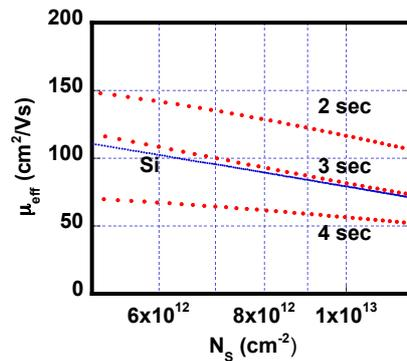
Fig. 4. Channel mobility of depletion-mode GeSn pMOSFETs for 2, 3, and 4 sec RIE channel thinned samples.
