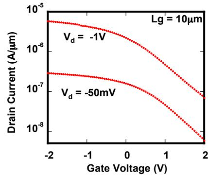
Fig. 2.  $I_d$ - $V_g$  characteristics of depletion-mode GeSn pMOSFETs with  $L = 10\mu\text{m}$  and drain voltage of -50 mV and -1V. The On/Off current ratio of 84 is obtained between  $V_g = -2$  and 2V at  $V_d = -1\text{V}$ .
