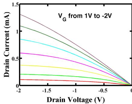
Fig. 3.  $I_d$ - $V_d$  characteristics of depletion-mode GeSn pMOSFETs with GeSn channel thickness of <10 nm for different gate voltages, showing clear channel control.
