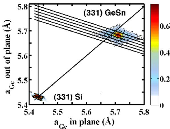
Fig. 1 XRD reciprocal space map around the (331) reflection of 37 nm crystallized GeSn (sample C, 4.5% Sn/(Sn+Ge) flux ratio), transformed to in-plane and out-of-plane lattice spacings. The color bar indicates the XRD intensity (arbitrary units) in log scale.
