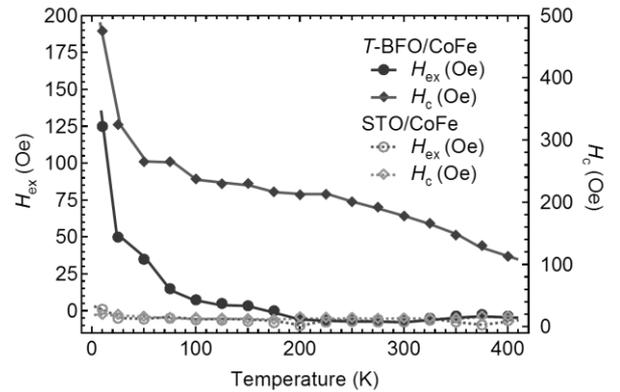
Fig. 5 Temperature dependence of  $H_{ex}$  and  $H_c$  for *T*-BFO/CoFe bilayer
