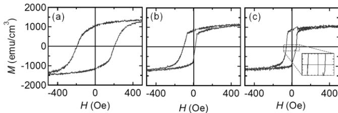
Fig. 3 Magnetization curves of (a)*T*- and (b),(c) *R*-BFO/CoFe bilayers measured at 300 K
