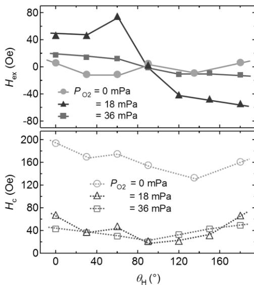
Fig. 4 Applied magnetic field angle dependence of  $H_{ex}$  and  $H_c$  for BFO/CoFe bilayers.
