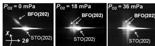
Fig. 2 XRSM images of BFO single layers.
