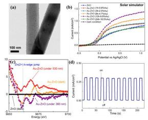
Fig. 3 (a) TEM image of the gold nanoparticles modified ZnO nanowires. (b) I-V curves of the ZnO nanowires with/without loading of gold nanoparticles at 100 mW/cm<sup>2</sup>. (c) XAS measurement and (d) I-t curves of the ZnO nanowires with/without loading of gold nanoparticles at 530 nm monochromatic light.<sup>6</sup>
