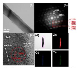
with CdTe QDs. (b) Corresponding electron diffraction pattern of (a). (c) HR-TEM micrograph of a ZnO nanowire decorated with CdTe QDs. (d) Elemental mapping images of the Zn, Cd, and Te, respectively.<sup>5</sup>
