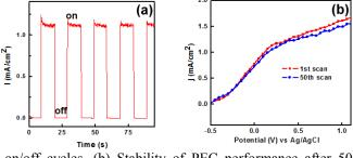
on/off cycles. (b) Stability of PEC performance after 50 scans.<sup>5</sup>
