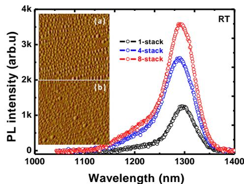
Fig. 1 RT PL spectra of the InAs/Sb:GaAs stacked QDs with different stacking number grown on Ge/Si substrate. The inset shows  $1 \times 1 \mu\text{m}^2$  AFM images of the first (a) and eighth (b) layer of the uncapped InAs/Sb:GaAs QDs.
