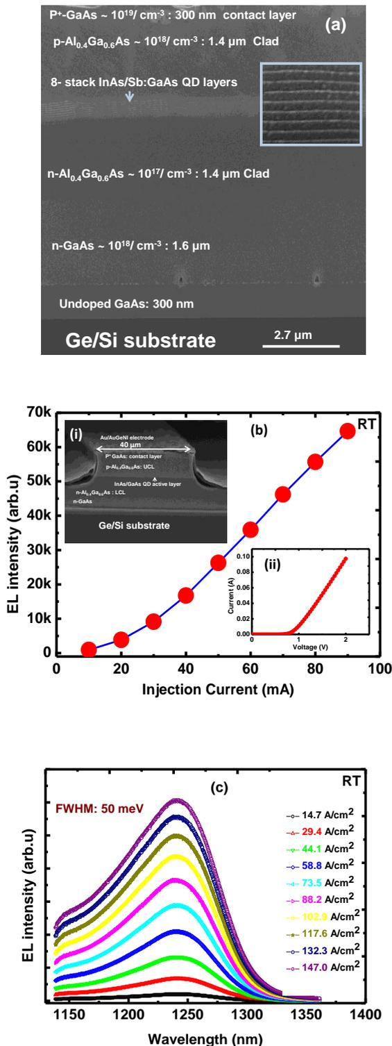
Fig. 2 (a) Cross-sectional HRSEM of the sample. The thickness and doping concentration of each layer is indicated. The inset shows a detailed image of the QD layers. (b) Light-current characteristics of the device [inset (i)] at RT. Inset (ii): plot of forward bias I-V characteristics of the diode. (c) EL spectra of the device at RT for different injection currents.
