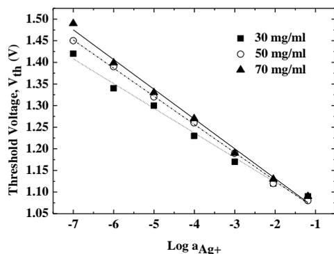
Fig. 3 Threshold voltages of  $Ag^+$ -EGFET sensor with 30 mg/ml, 50 mg/ml and 70mg/ml P3HT thin films in various  $Ag^+$  activities.
