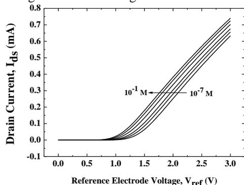
Fig. 2  $I_{ds}$ - $V_{ref}$  curves for  $Ag^+$ -EGFET sensor with 70 mg/ml P3HT thin film.
