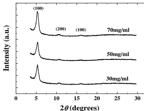
Fig. 4 X-ray diffraction (XRD) profiles of various concentrations P3HT films.
