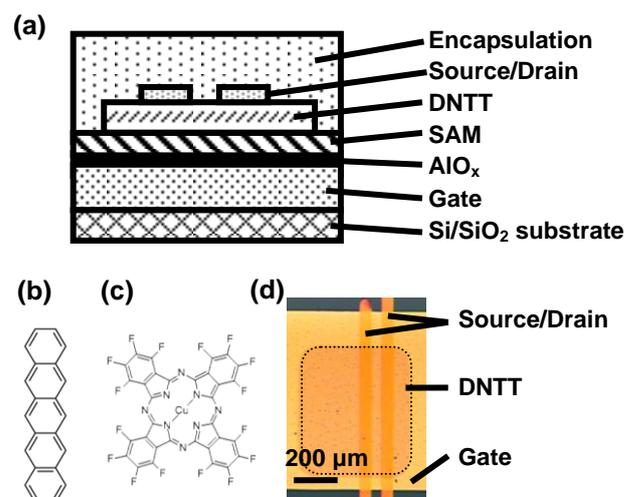
Fig.1. Device structure: (a) Cross section structure of OTFTs. (b), (c) Chemical structure of DNTT (b) and n-octadecyl phosphonic acid (c). (d) Optical image of OTFT without encapsulation from top view.
