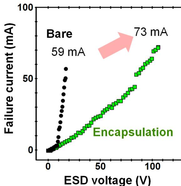
Fig.2 ESD failure current as a function of ESD voltage: Black dots shows organic TFTs without polymer encapsulation and organic TFTs with encapsulation is shown by light green dots.
