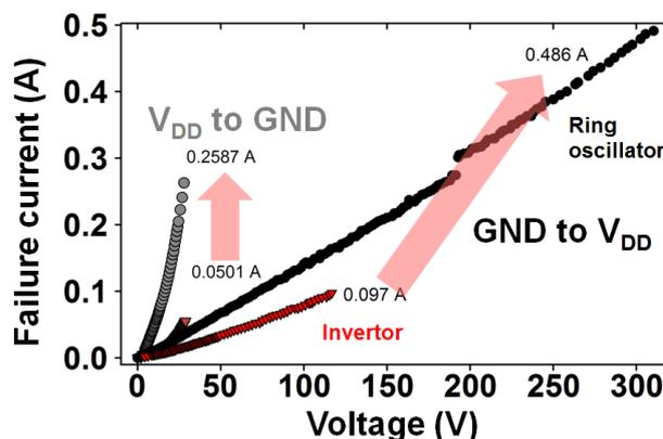
Fig.3 Failure current on organics RO and organic invertors as a function of ESD voltage: Black and red dots shows data with a ESD path from GND to  $V_{DD}$ , and gray and light red dots shows data with the path from  $V_{DD}$  to GND. In each ESD direction, RO flows 5 times larger failure current than inverter. Invertors are prepared in isolation from ROs
