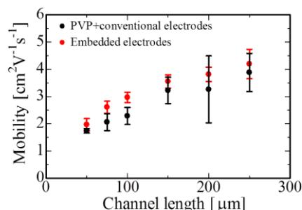
**Fig. 4.** Channel length vs. field-effect mobility of top-gate C<sub>8</sub>-BTBT FETs with embedded electrodes and conventional electrodes prepared on PVP buffer layers.
