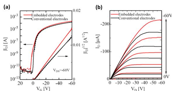
**Fig. 3.** (a) Transfer and (b) output characteristics of top-gate C<sub>8</sub>-BTBT FETs with embedded and conventional electrodes. Channel length is 250 μm.
