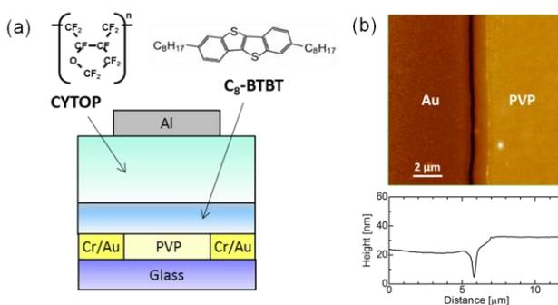
**Fig. 1.** (a) Device structure of top-gate C<sub>8</sub>-BTBT FETs with embedded source-drain electrodes. (b) AFM image and height profile of a fabricated substrate with embedded electrodes
