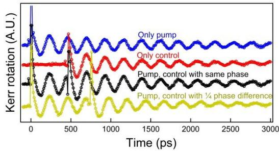
Fig. 1 Time evolution of the Kerr rotation in a CdTe QW sample observed with pump alone (blue curve), control alone (red curve), pump and control with the same phase (black curve), pump and control with a quarter phase difference (yellow curve) as  $\sigma^+$  circularly polarized pulses.
