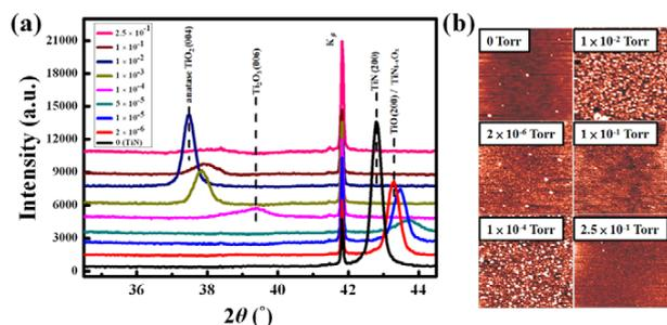
Fig. 1 (a) The XRD pattern of samples deposited with various oxygen pressures. (b) Surface morphologies of samples measured by AFM.
