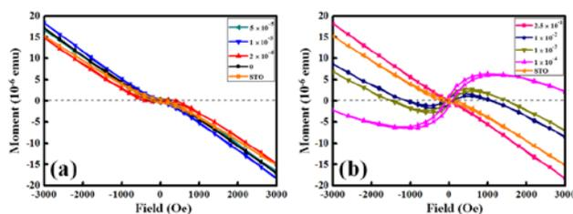
Fig. 2 *M-H* curves measured by SQUID at room temperature (300 K) for the STO substrate and the samples deposited at  $P_{O_2}$  (a) from 0 to  $5 \times 10^{-5}$  torr, (b) from  $1 \times 10^{-4}$  to  $2.5 \times 10^{-1}$  torr.
