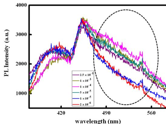
Fig. 3 The photoluminescence spectrum of TiNO samples
